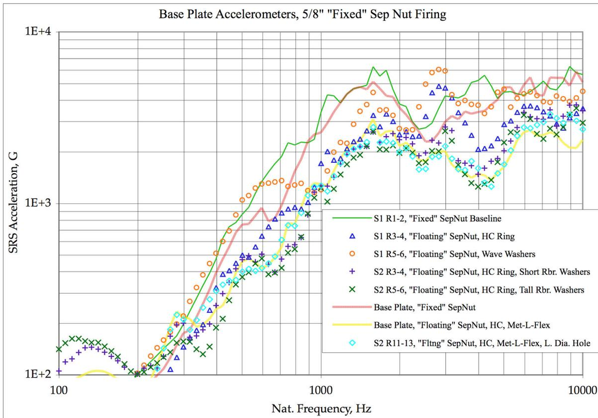
Figure 5. SRS Data Envelopes for Multiple Sep Nut Configurations on Simple Plate
