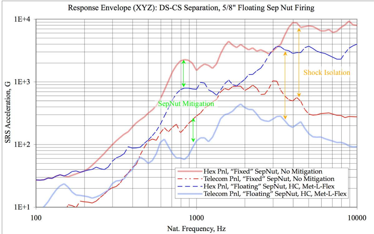
Figure 9. DS Telecom Configuration, Shock Attenuation at Telecom Plate
