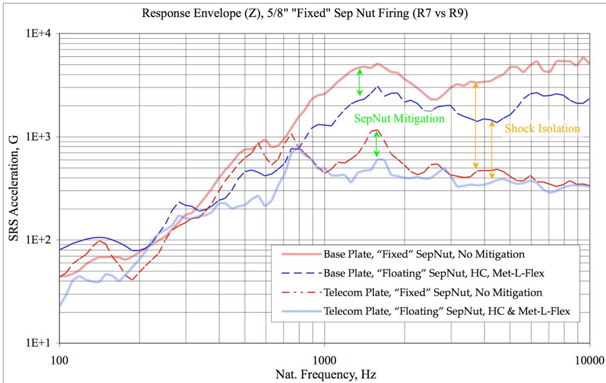
Figure 6. Shock Attenuation at Telecom Plate
