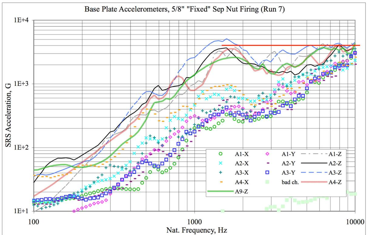
Figure 4. SRS Data for "Fixed" Sep Nut Firing on Simple Plate
