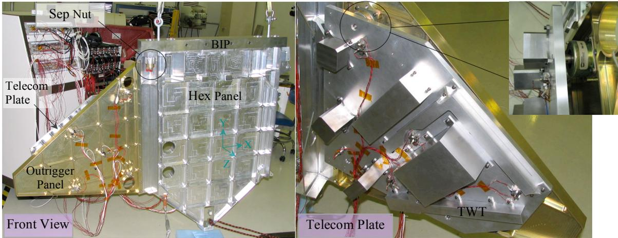
Figure 7. Descent Stage Hex and Outrigger Panel Assembly, Telecom Test Configuration
