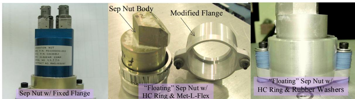
Figure 3. “Fixed” versus “Floating” Sep Nut Configurations
