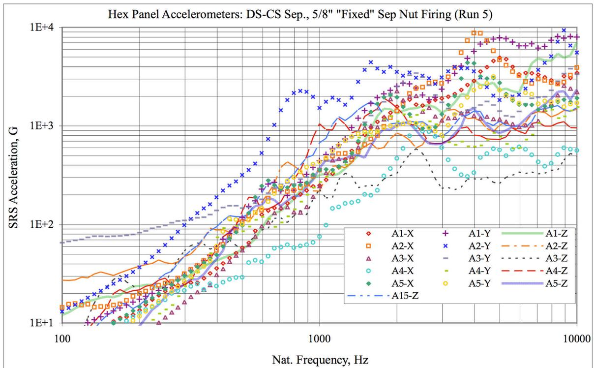
Figure 8. SRS Data for “Fixed” Sep Nut Firing on DS Hex Panel
