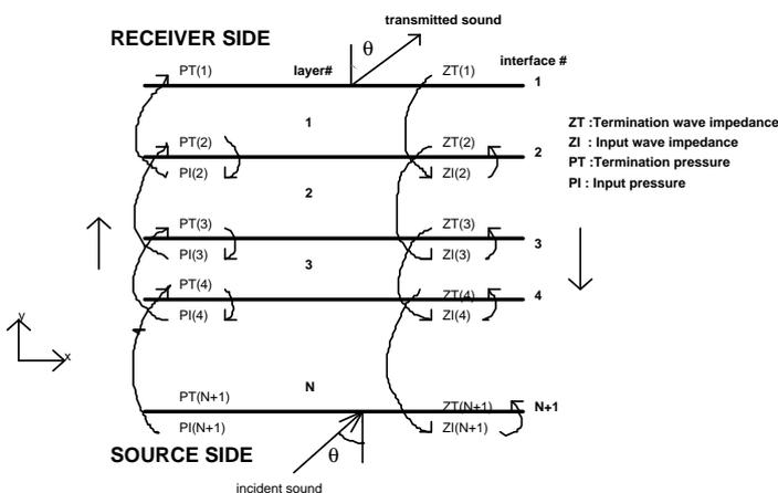
Figure 1. Calculation process of the impedance model for multi-layered elements (Arrows indicate the order of computations)
