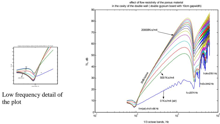
Figure 9. Variation of the narrow band sound transmission losses of double gypsum wall with 0.10m cavity (infinite size).
