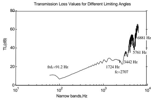
Figure 3. Predicted narrow band TL for a multilayered structure by using the infinite model MULAY and the calculated modes according to the basic theories. (Double gypsum board with 10 cm airgap)
