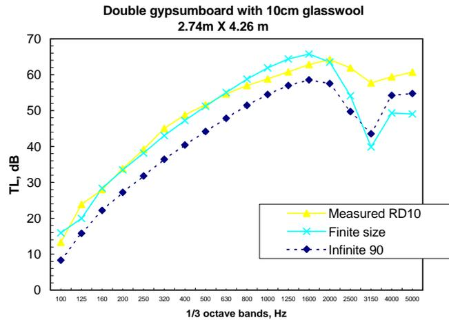
Figure 6. Comparison between the measured and calculated data for double gypsum board with 10 cm glasswool in large size: 2.74 m X 4.26m
