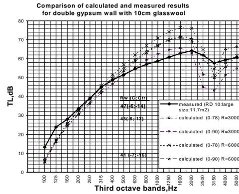
Figure 4. Comparison of calculated (as infinite) and the measured results for double gypsum board with 10cm glasswool ( R: flow resistivity, angles of incidence are shown in the legend) [1]
