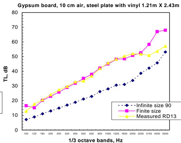
Figure 8. Comparison between the measured and calculated data for a multilayered structure in small size: 1.21 m X 2.43 m.
