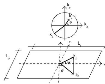
Figure 2. Wave parameters in windowing technique [4]. a) Wave number components contributing to radiated power in solid angle. b) Parameters relative to incident wave on a finite element.
