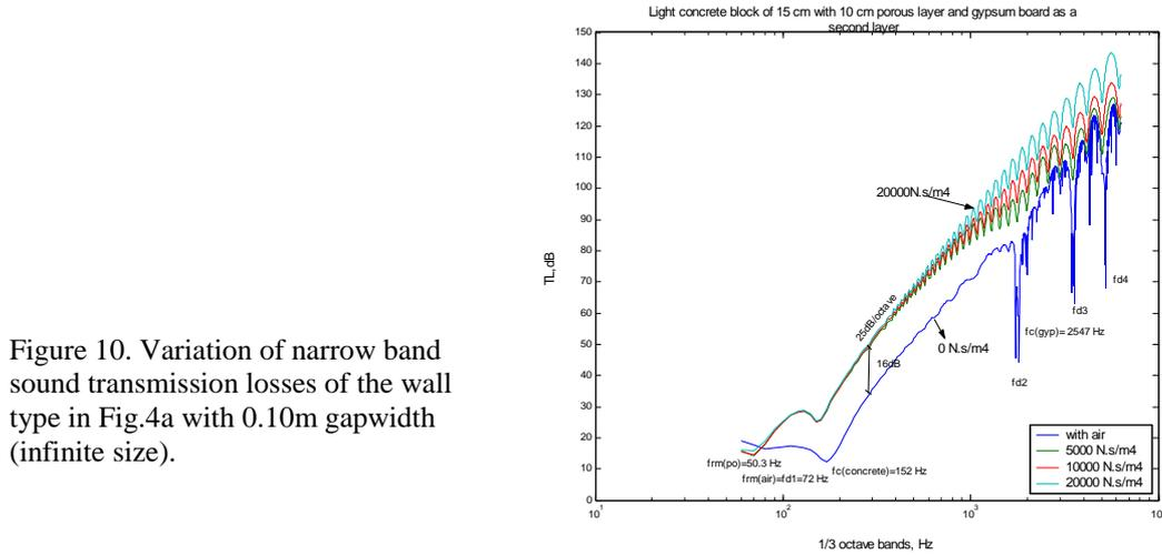
Figure 10. Variation of narrow band sound transmission losses of the wall type in Fig.4a with 0.10m gapwidth (infinite size).
