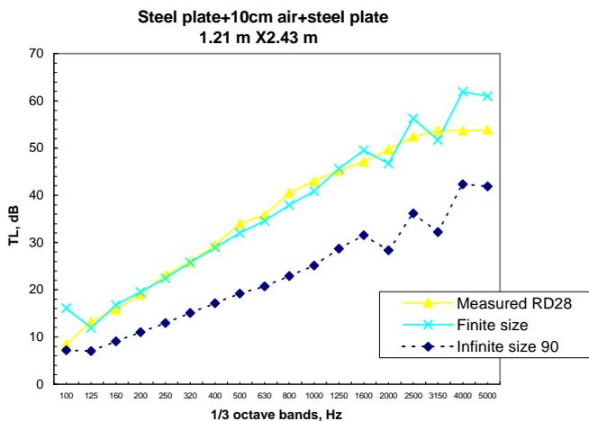
Figure 7. Comparison between the measured and calculated data for double steel plates with 10 cm air in small size: 1.21 m X 2.43 m
