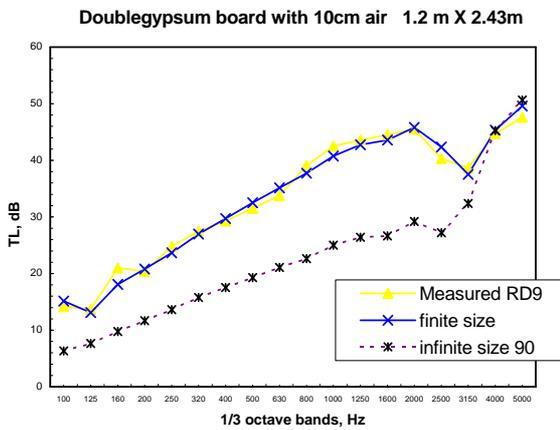
Figure 5. Comparison between the measured and calculated data for double gypsum board with 10cm air in small size: 1.2 m X 2.43m
