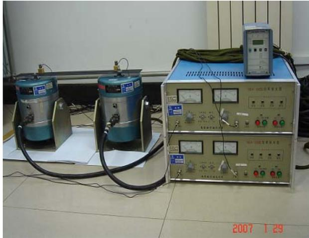
Figure 4. Two small shakers and power amplifier
