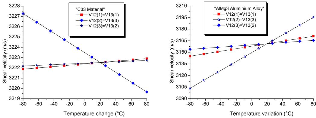
**Figure 3.** Shear velocity as function of temperature variations for C33 and AlMg3 Materials
