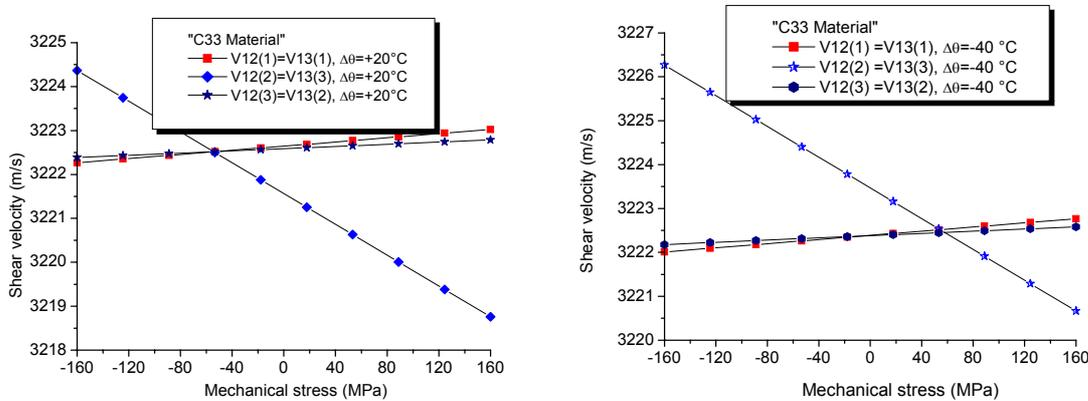
**Figure 5.** Shear velocity as function of the applied mechanical traction and compression stresses under temperature variations  $\Delta\theta = 20^\circ\text{C}$  and  $\Delta\theta = -40^\circ\text{C}$ . Case of C33 Material.
