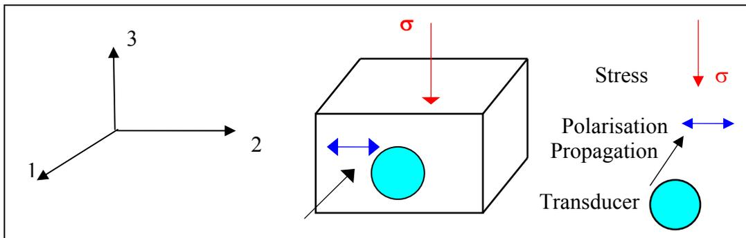
**Figure 1.** Loading mode and wave propagation with regard to the referential of the sample
