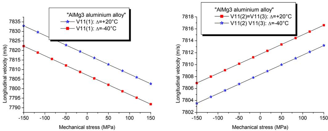
**Figure 6.** Longitudinal velocity as function of the applied mechanical traction and compression stresses under temperature variations  $\Delta\theta = 20^\circ\text{C}$  and  $\Delta\theta = -40^\circ\text{C}$ . Case of AlMg3 Material.
