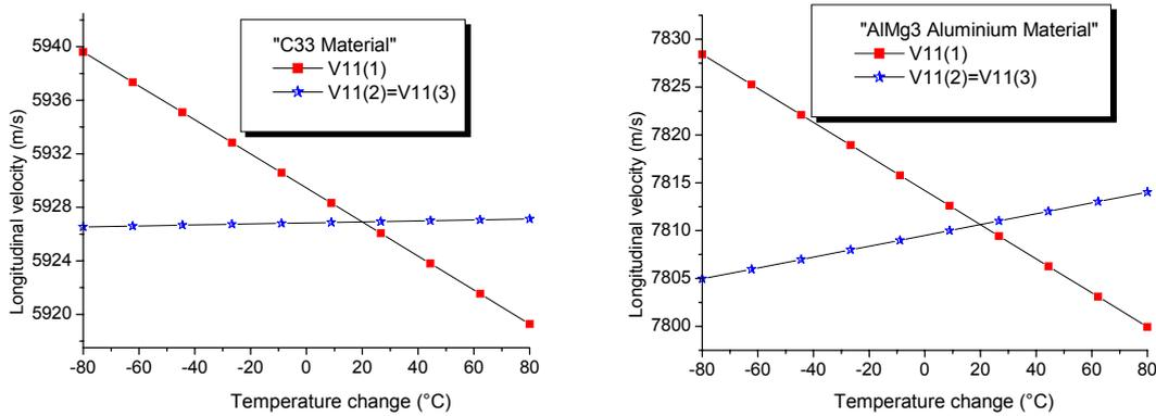
**Figure 2.** Longitudinal velocity as function of temperature variations for C33 and AlMg3 Materials.
