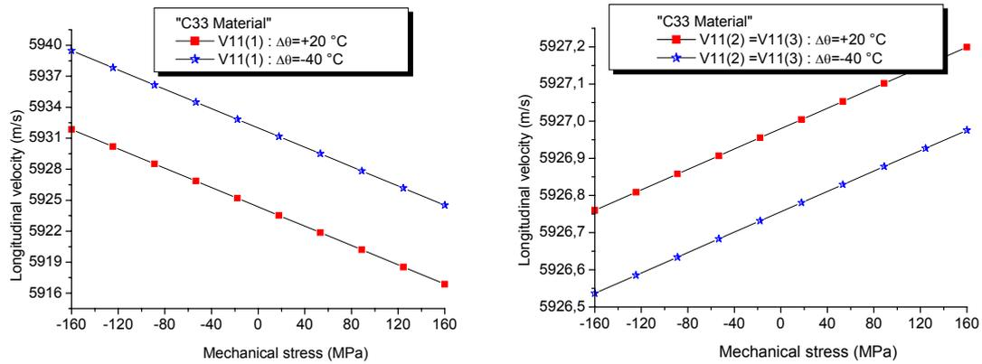
**Figure 4.** Longitudinal velocity as function of the applied mechanical traction and compression stresses under temperature variations  $\Delta\theta = 20^\circ\text{C}$  and  $\Delta\theta = -40^\circ\text{C}$ . Case of C33 Material.
