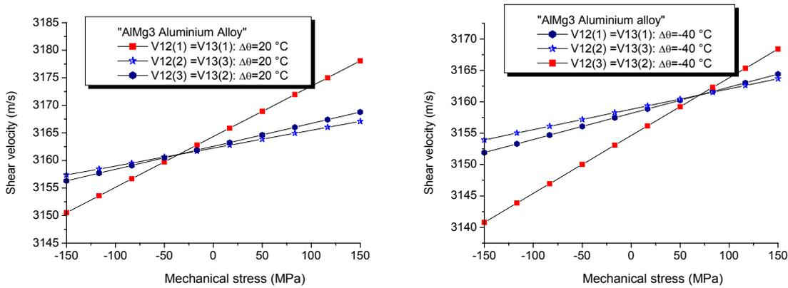
**Figure 7.** Shear velocity as function of the applied mechanical traction and compression stresses under temperature variations  $\Delta\theta = 20^\circ\text{C}$  and  $\Delta\theta = -40^\circ\text{C}$ . Case of AlMg3 Material
