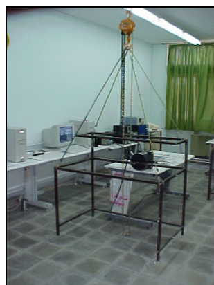
Figure 9. Modal test of 3D steel structure.
