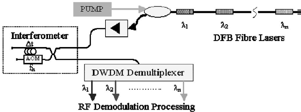
Figure 4: Multiplexed fibre laser array system.
