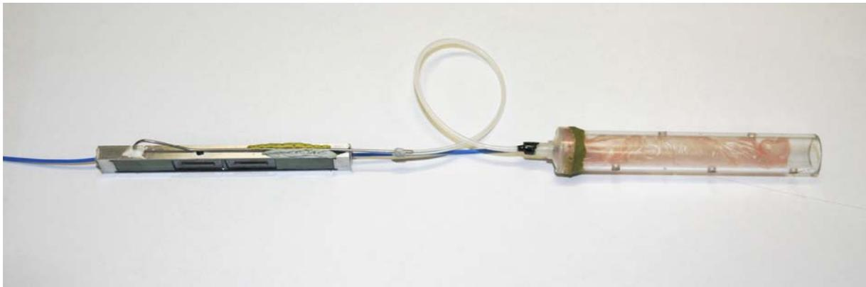
Figure 6: Pressure compensated fibre laser hydrophone showing acoustic transducer (containing fibre laser) (left) and external bladder (right).
