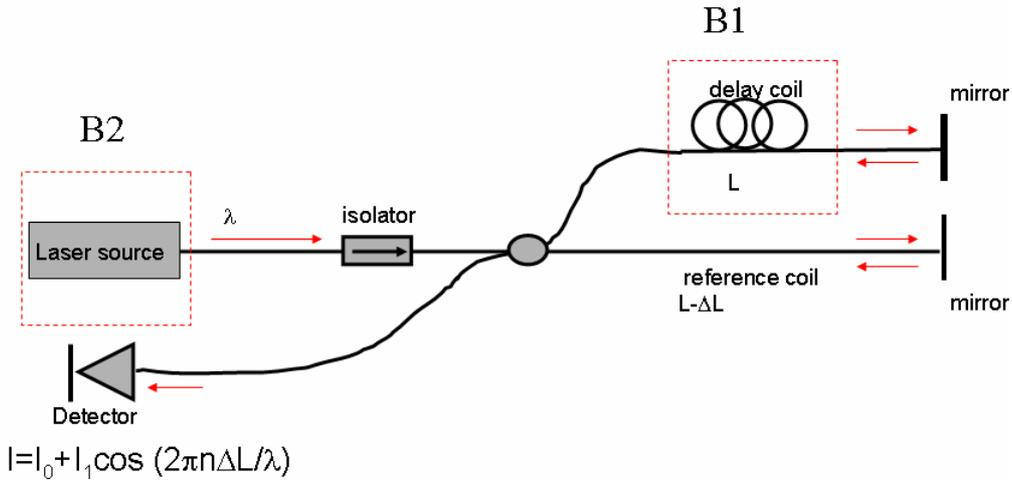
Figure 1: Michelson fibre interferometer illustrating the principle of fibre optic acoustic sensing. In calculating the path length in each arm the total transit distance of the light “beam” must be taken into account. Thus, for a reflective geometry such as shown here, the path imbalance  $\Delta L$  is twice the difference in fibre lengths between the two arms. Similarly, the coil path length  $L$  is twice the actual length of fibre in the coil.
