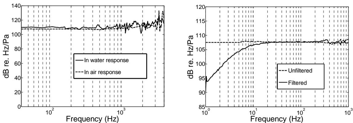
Figure 5: a) Acoustic response of fibre laser hydrophone; b) low frequency response of pressure compensated hydrophone showing roll-off below 20Hz.
