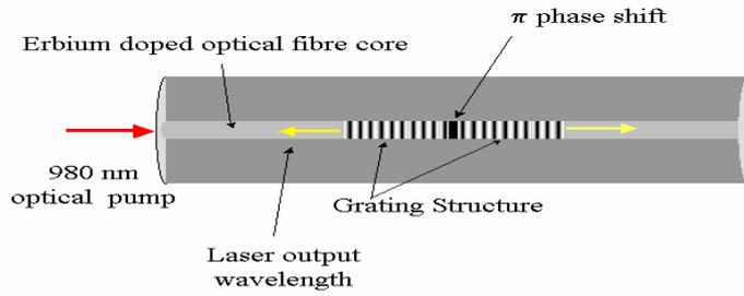
Figure 3: A Distributed feedback fibre laser.
