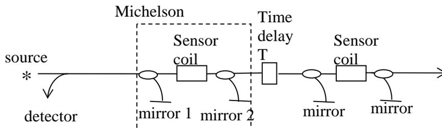
Figure 2: Outline of a serial Michelson geometry suitable for time domain multiplexing.
