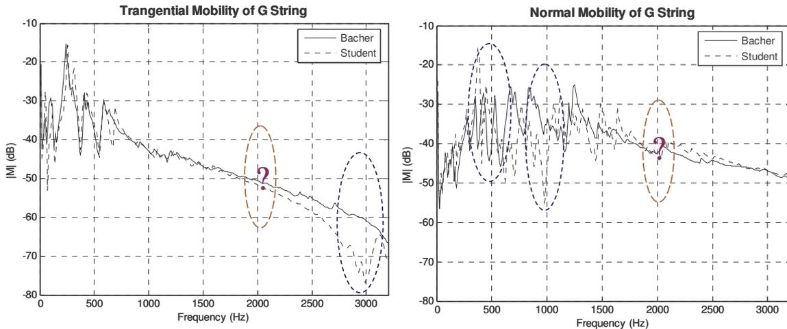
Figure 8. Measured tangential and normal mobility functions of at the G string location of the two violins.
