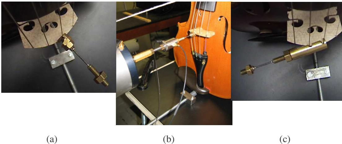
Figure 7. Mobility measurement experimental set-up and a connector between impedance head and the string on the bridge. (a) connector for normal mobility, (b) mini-shaker, impedance head and connector, (c) connector for tangential mobility.
