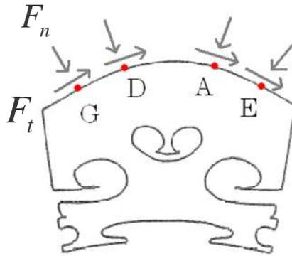
Figure 6. Tangential and normal forces at G string location of the bridge.
