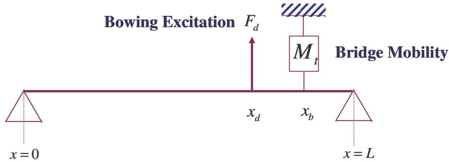
Figure 10. Simple string and bridge mobility model for studying bowing sensitivity.
