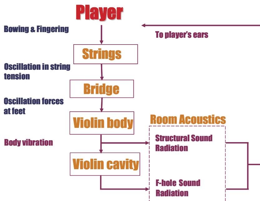
Figure 1 Flow diagram of production of violin sound.
