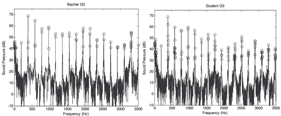
Figure 3. PSD of G3 (196 Hz) of Bacher and student violins. Little circles in the figures are the identified peaks in the narrow frequency spectrum. The circle with largest value in a major peak is used to represent the peak value of the fundamentals and overtones.
