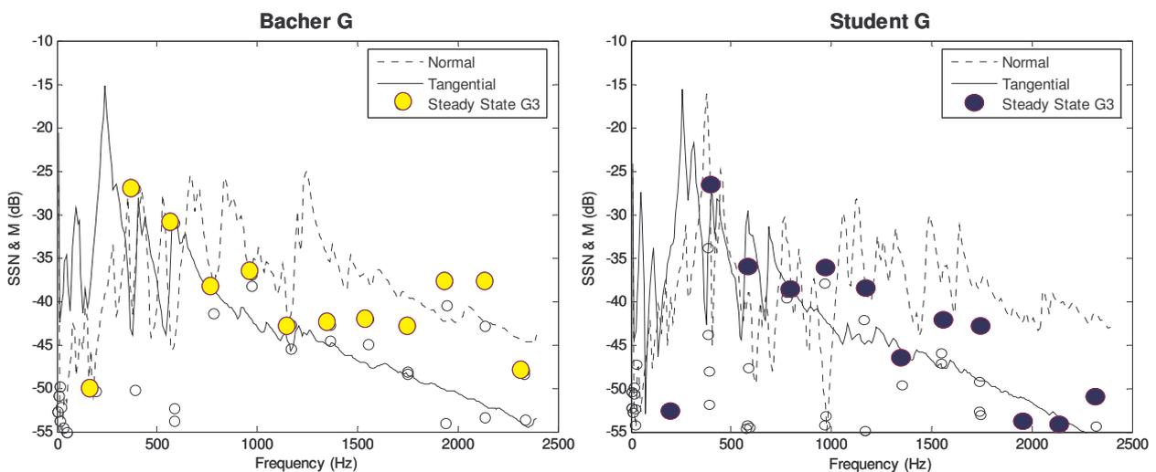
Figure 9. Measured tangential and normal mobility functions of at the G string location of the two violins.
