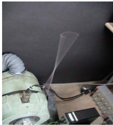
Figure 4 – One to one internal resonance of the circular cantilever beam on the second mode
