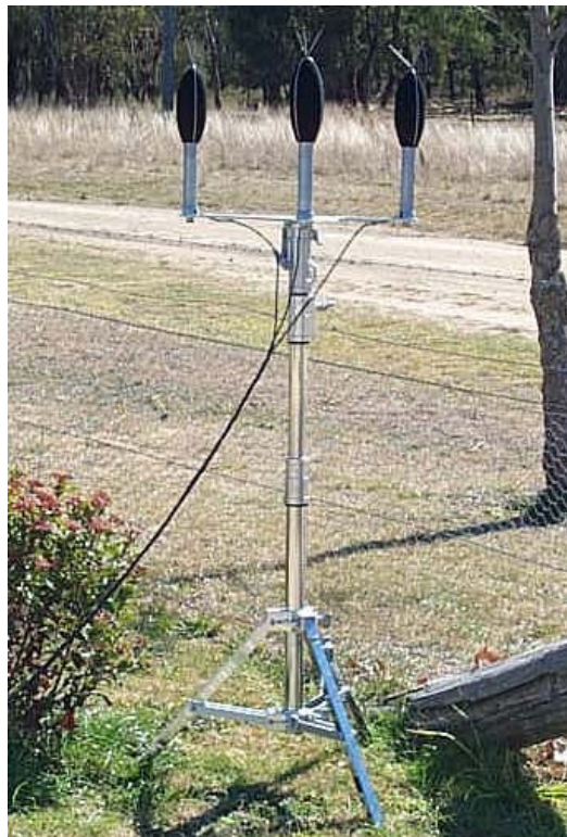
Figure 1 Typical Field Microphone Setup
