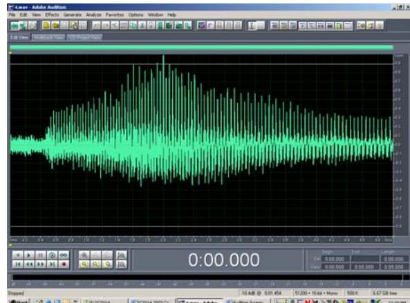
Figure 4. Unacceptable Engine Brake RMS = 4.73
