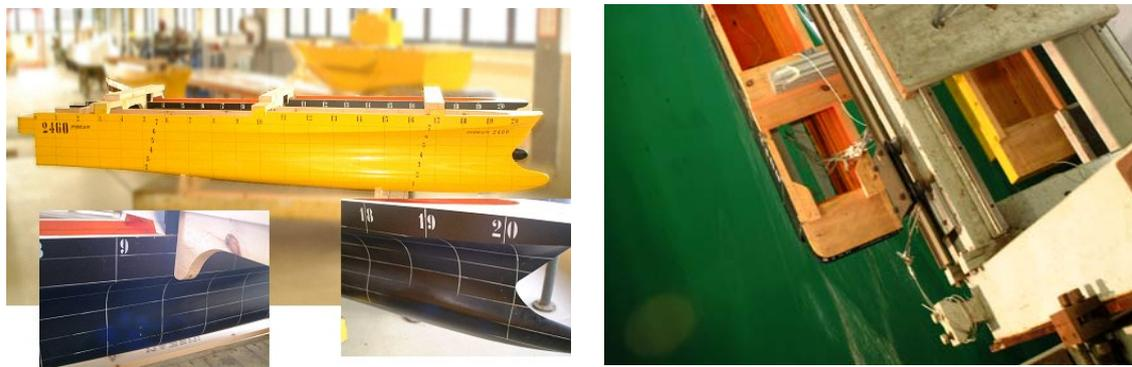
Figure 1 Catamaran model and test sections for pressure measurements
