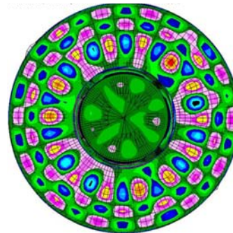
Figure 3: Mode shape (28,3) at 577.34 Hz
