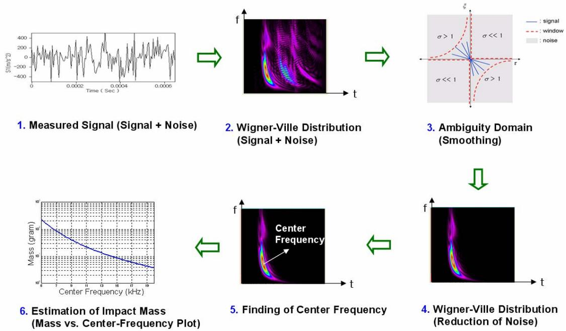
Figure 4. Proposed method for impact mass estimation.
