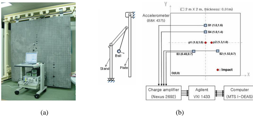
Figure 5. Experimental setup for impact mass estimation: (a) View of the experimental setup, (b) Schematic of the experimental setup, where the locations of two impact point (p1 and p2) and four accelerometers (S1, S2, S3 and S4) are indicated.
