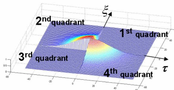
Figure 3. An asymmetric exponential window for removing the noise components located inside the 1<sup>st</sup> and 3<sup>rd</sup> quadrants in an ambiguity function domain.
