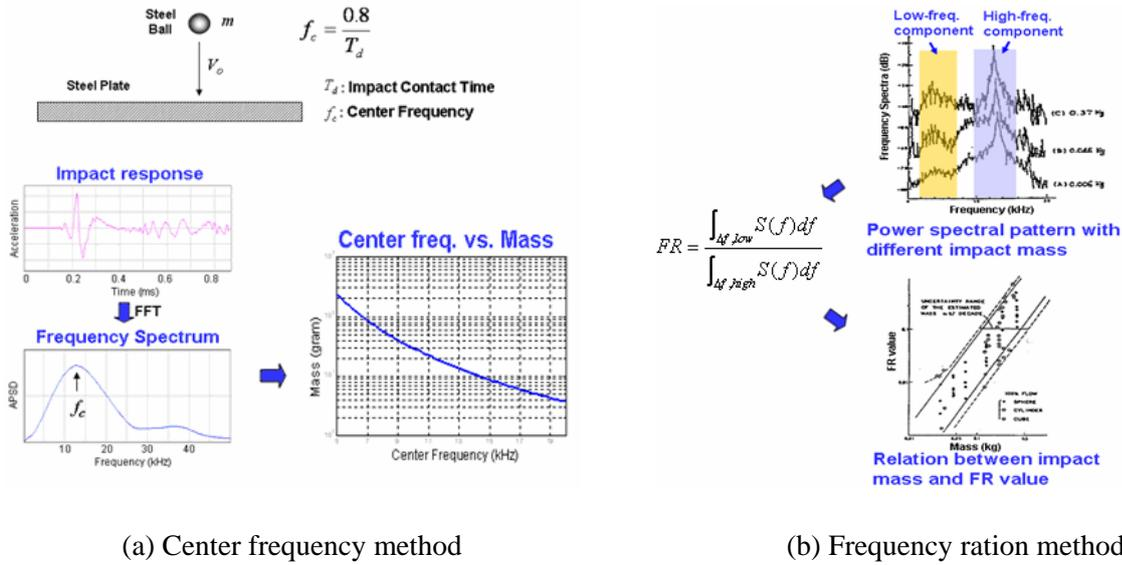
Figure 1. Conventional mass estimation technique.
