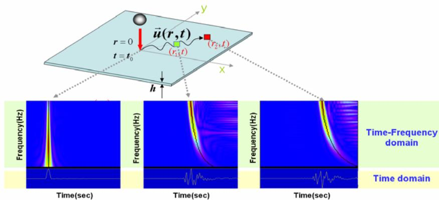
Figure 2. Wave propagation due to impact: dispersive flexural wave component is represented as a curved line with a negative slope in the time-frequency domain.
