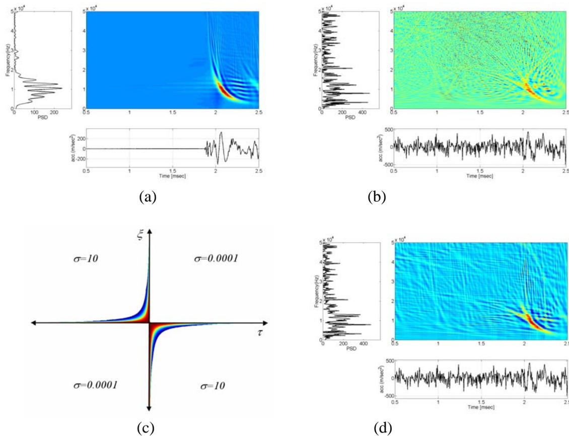
Figure 6 Time-frequency analysis results that demonstrate the noise rejection capability:
