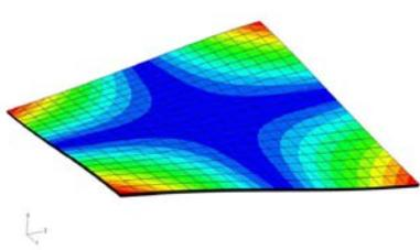
Figure 8: The first mode shape of Plate C (70.07 Hz)
