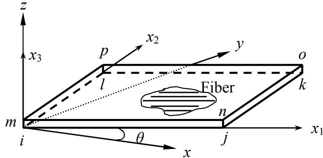
Figure 1: The cross-ply laminated plate and the coordinate system.
