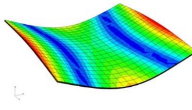
Figure 9: The second mode shape of Plate C (132.71 Hz)
