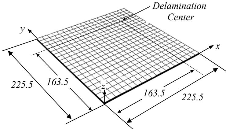
Figure 2: The finite element model of the laminated plate and the delamination region center.
