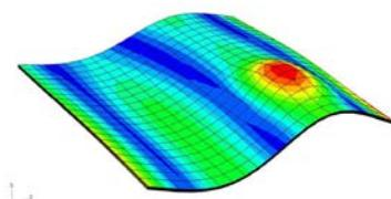
Figure 14: The seventh mode shape of Plate C (370.37 Hz).
