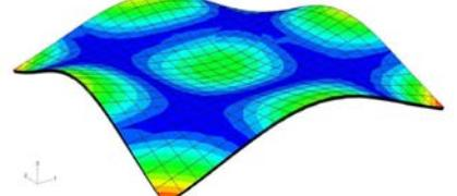
Figure 13: The sixth mode shape of Plate C (357.12 Hz).
