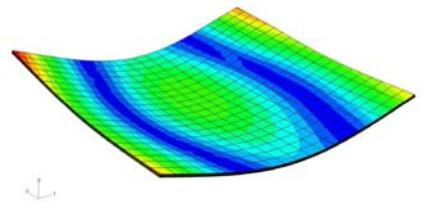
Figure 10: The third mode shape of Plate C (166.71 Hz)
