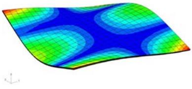
Figure 11: The fourth mode shape of Plate C (194.53 Hz).
