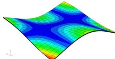
Figure 12: The fifth mode shape of Plate C. (216.15 Hz)
