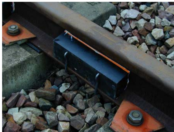
Figure 13. Discrete form of rail dampers applied at SNCF test site [49].
