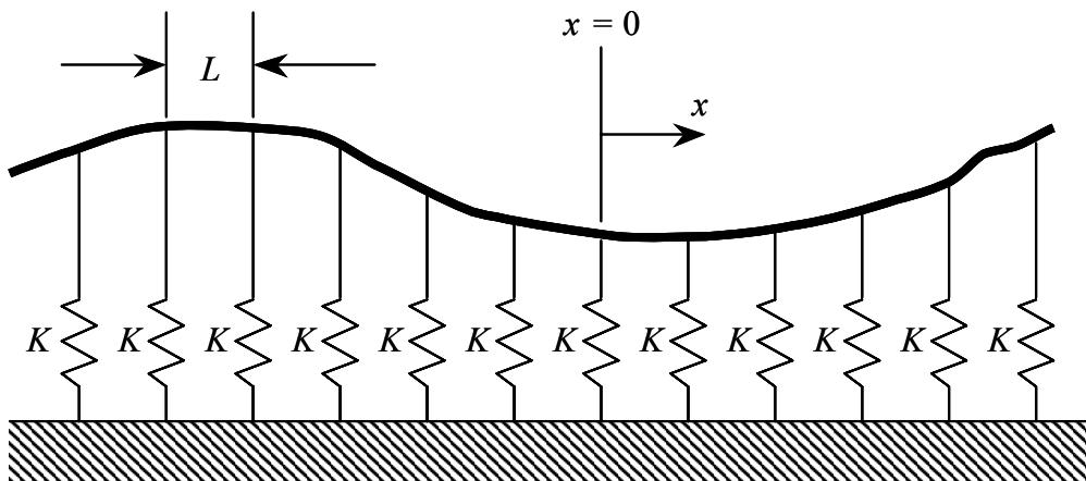
Figure 1. Tensioned and reinforced string with coordinate system
