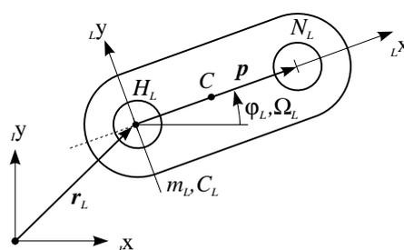
Figure 1: Kinematic of a Link
