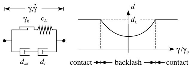
Figure 2: Force Element and Characteristic of Damping
