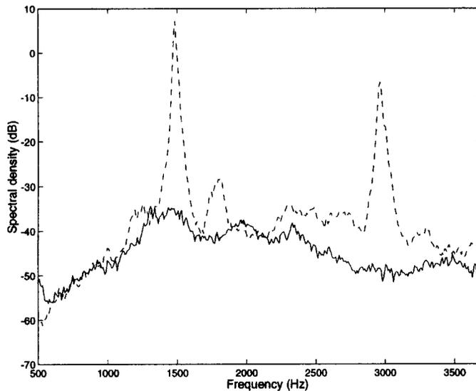
Figure 4: The spectral density of tool vibration with 20 tap FIR filter feedback control (solid) and without (dashed). Cutting speed  $v = 80$  m/min, cut depth  $a = 0.9$  mm, feed rate  $s = 0.25$  mm/rev, tool DNMG 150604-PF, grade 4015.
