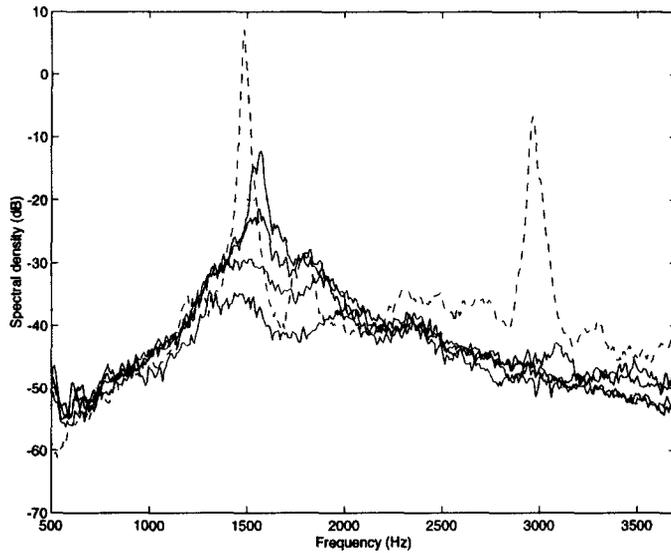
Figure 5: The spectral densities of tool vibrations with 20 tap FIR filter feedback control and four different leakage factors (solid) and the spectral density without feedback control (dashed). Leakage factors  $\gamma = 1, 0.9999, 0.999, 0.99$ , cutting speed  $v = 80$  m/min, cut depth  $a = 0.9$  mm, feed rate  $s = 0.25$  mm/rev, tool DNMG 150604-PF, grade 4015.
