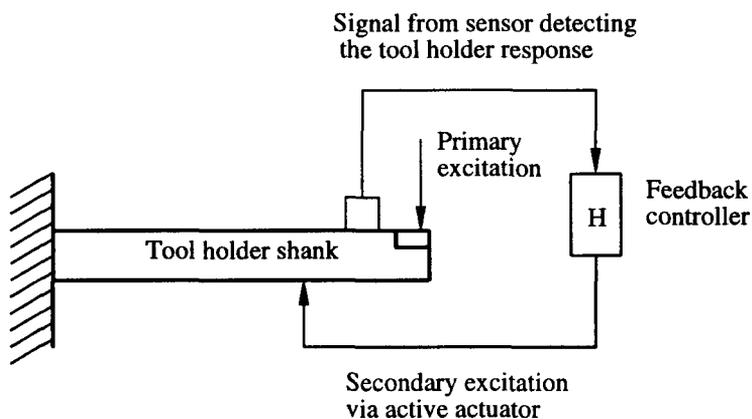
Figure 1: A machine-tool feedback control system[1].
