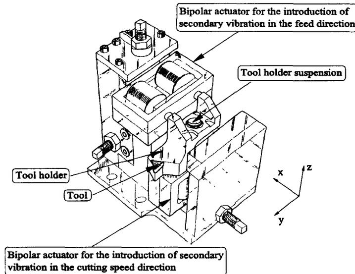
Figure 2: Tool holder with integrated actuators for the control of tool vibrations in the metal cutting process [7].
