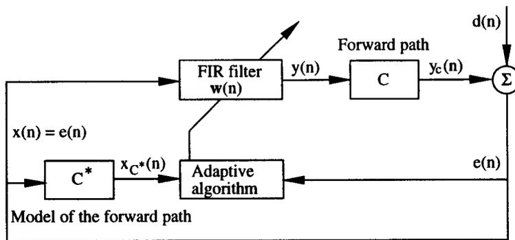
Figure 3: Equivalent block diagram of the feedback control situation with the filtered-x LMS algorithm[1].
