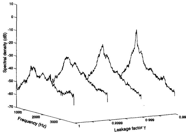
Figure 6: The spectral densities of tool vibrations with 20 tap FIR filter feedback control and four different leakage factors. Leakage factors  $\gamma = 1, 0.9999, 0.999, 0.99$ , cutting speed  $v = 80$  m/min, cut depth  $a = 0.9$  mm, feed rate  $s = 0.25$  mm/rev, tool DNMG 150604-PF, grade 4015.
