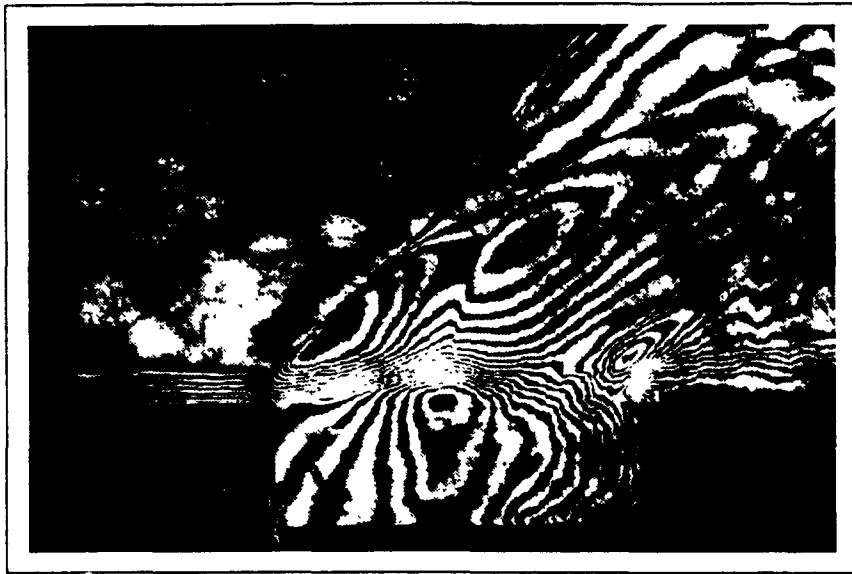
Figure 10 Experimental Interferogram showing shear layer impingement M_{\infty}=1.5 Zhang and Edwards 15 .
