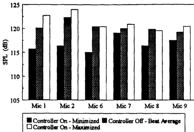
Figure 5. Cabin SPL corresponding to the arrangement of Fig.4 (from Ref. 8)
