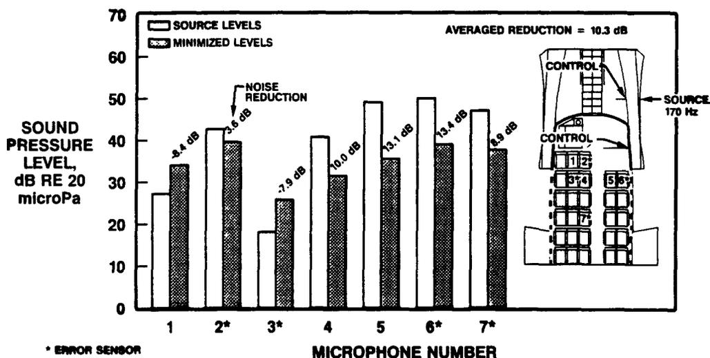
Figure 7. Cabin SPL corresponding to the system of Fig.6 (from Ref. 12)
