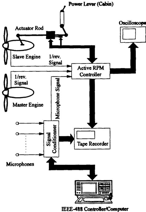
Figure 4. Experimental setup used by Pla *et al* in synchrophasing tests (from Ref. 8)
