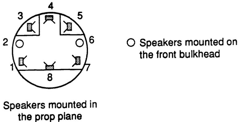
Figure 2. Locations of active speakers in the propeller plane of flight tests of Elliott *et al* (from Ref. 3)
