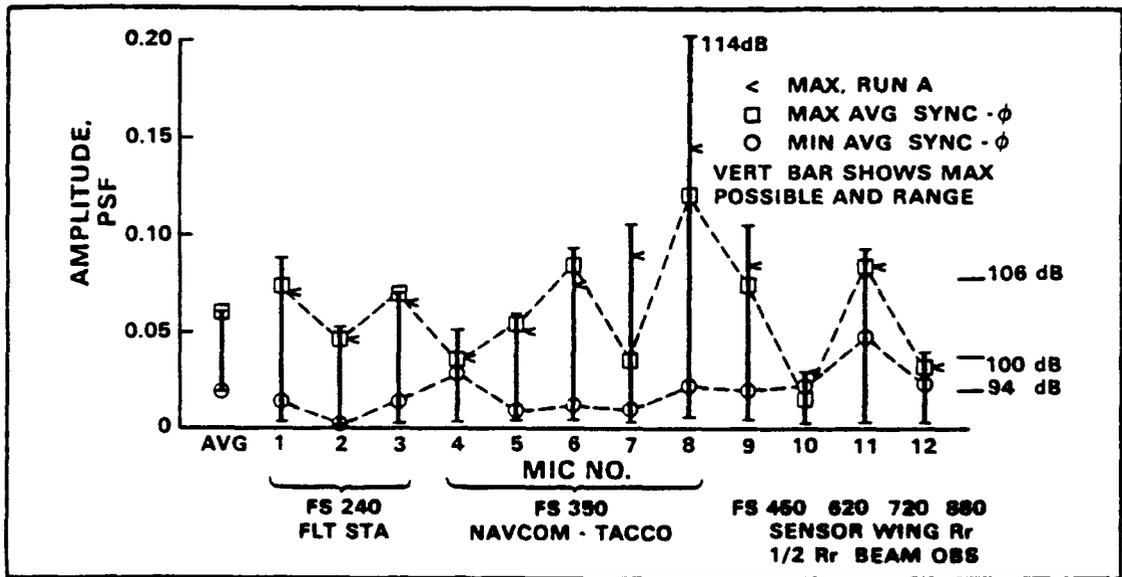
Figure 1. Predicted reduction of interior noise for various synchrophase angles (from Ref. 1)
