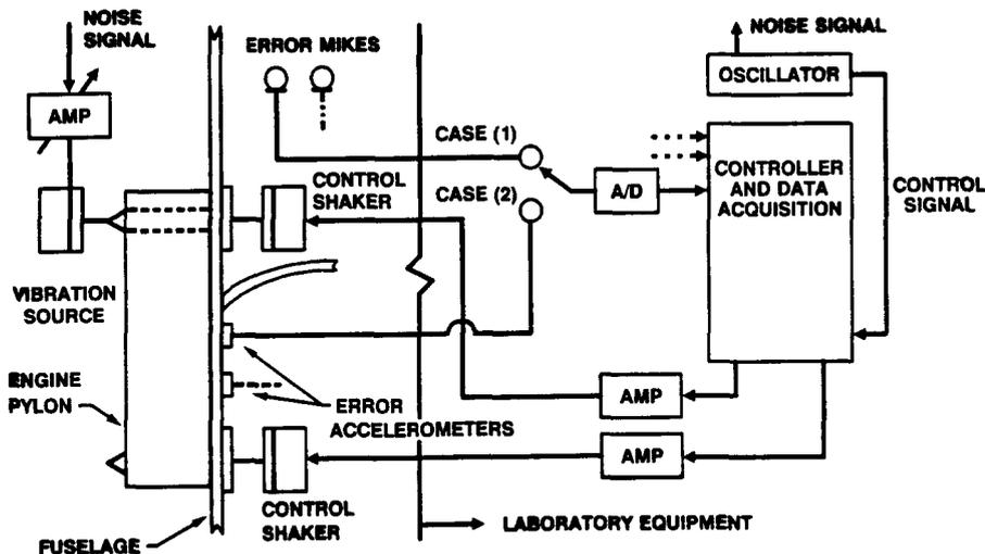
Figure 6. Experimental arrangement used by Simpson *et al* (from Ref. 12)
