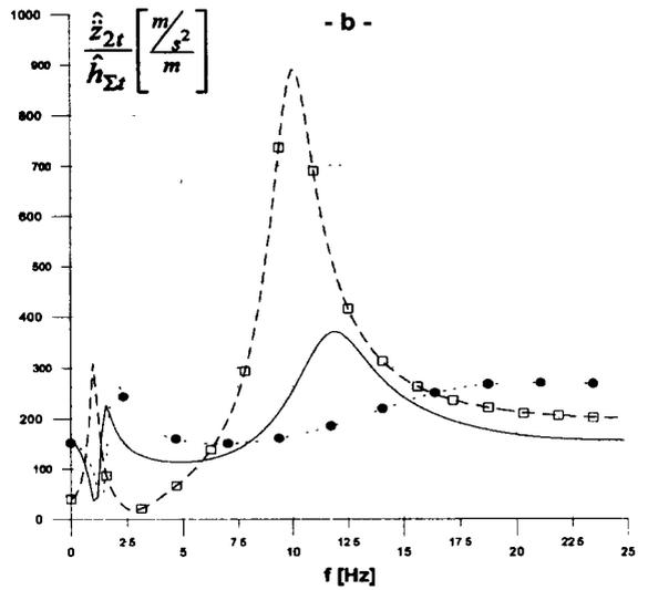
Fig 2. Reinforcement function for vertical accelerations in: a) the front part of bodywork, b) the rear part of bodywork.
