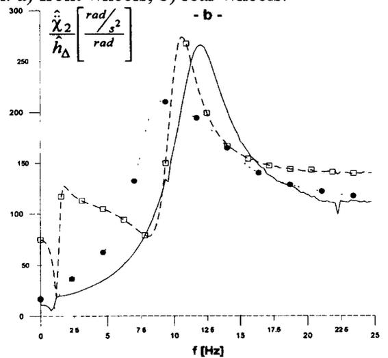
Fig 4. Reinforcement function for angular accelerations of: a) longitudinal tilts in bodywork, b) lateral tilts in bodywork.
