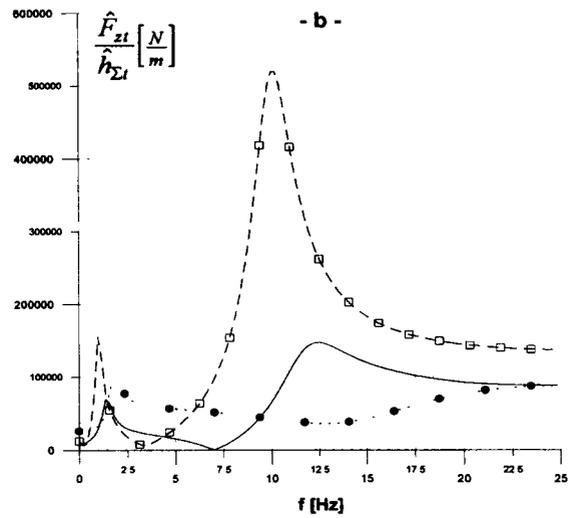
Fig 3. Reinforcement function for dynamic loads in: a) front wheels, b) rear wheels.
