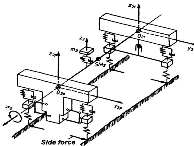
Fig 1. Analytical model of a vehicle where suspension has been considered.
