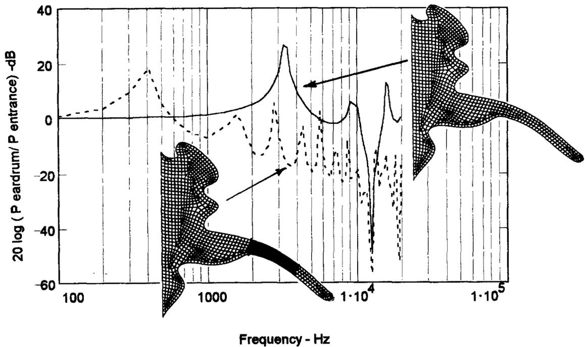
Figure 8: Eardrum SPL response for 2-D model for real ear with and without an ear plug
