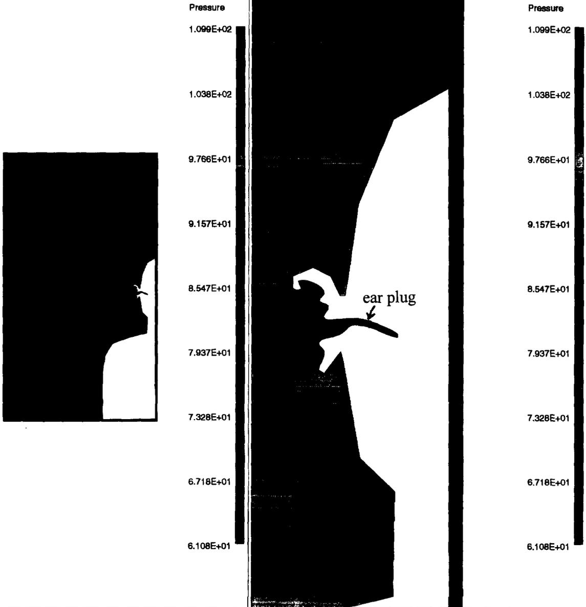
Figure 10: The eardrum SPL response for 2-D model for real ear canal, head and shoulders for plugged ear at 5KHz.
