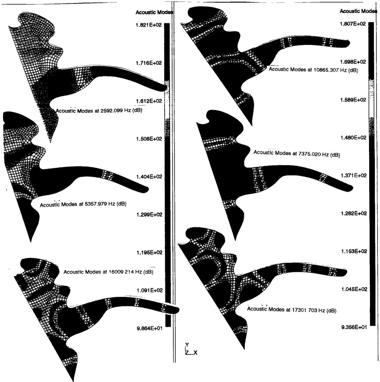
Figure 5: Acoustic resonance frequencies and mode shape of the pinna
