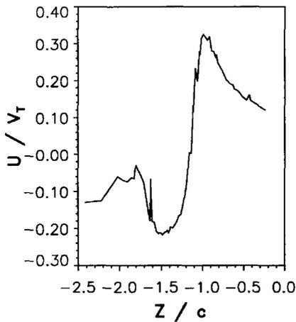
**Fig. 3.29 Radial velocity profiles through the vortex core near  $\Psi = 300^\circ$  (retreating side) and  $r/R = 0.8$  for moderate speed descent case**
