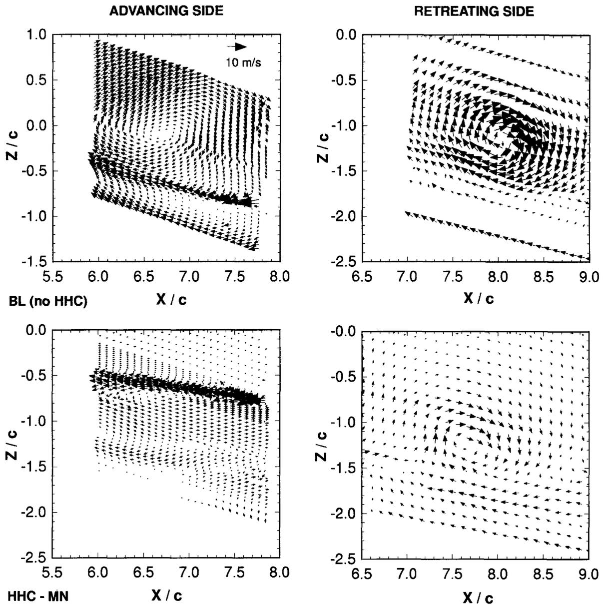
Fig. 3.28 Velocity fields in the vicinity of the blade tip for baseline case and minimum noise case for conditions of moderate speed descent on the advancing and the retreating sides
