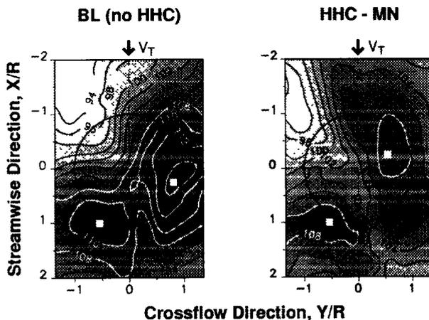
Fig. 3.21 shows the radiated acoustic field under the rotor for a simulated moderate speed (33 m/s)  $6^\circ$ -descent flight without (left) and with (right) the application of a 3-per-rev HHC with an optimum phase and amplitude input. Obviously, the BVI impulsive noise maximum under the advancing side is drastically reduced (by about 6 dB).
