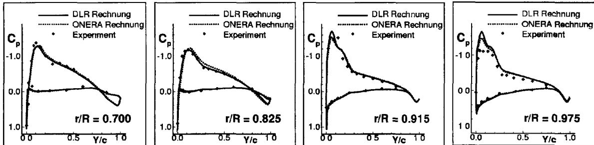
**Fig. 3.16** Comparison of predicted and measured surface pressure coefficients
