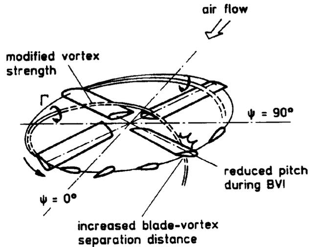
**Fig. 3.20 Noise reduction mechanism by Higher Harmonic rotor Control**
