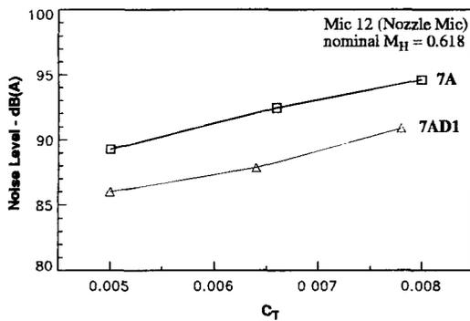
Fig. 3.12 Comparison of in-plane A-weighted levels for 7A and 7AD1 rotor at hover as function of thrust setting
