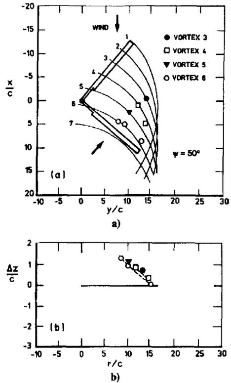
Fig. 3.8 Measured vortex section for moderate speed descent: (a) plan view comparing measurement and (prescribed) wake prediction for blade fixed at 50° azimuth, (b) side view showing measured separation distances
