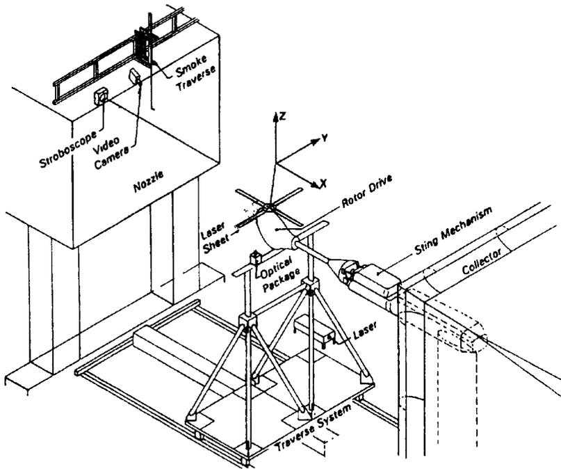
**Fig. 3.5 Test set-up for flow visualisation with the Laser Light Sheet technique**
