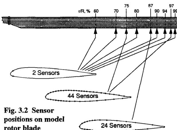
**Fig. 3.2 Sensor positions on model rotor blade**
