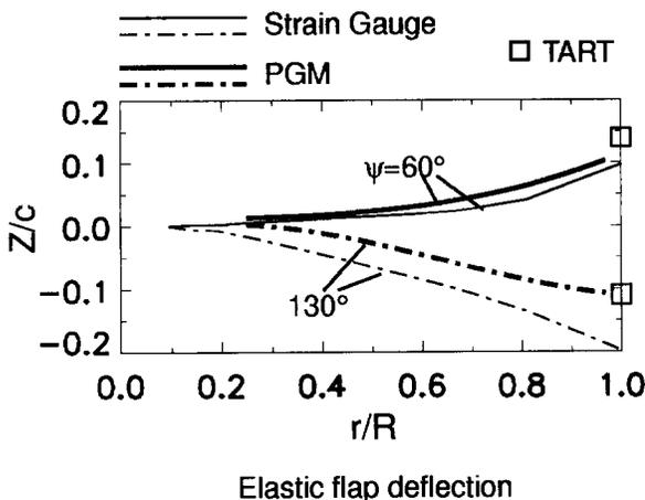
**Fig. 3.25 Elastic flap deflections as determined through the projected Grid Method**
