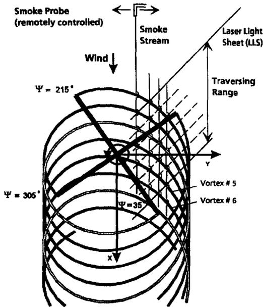
Fig. 3.7 Application of the Laser Light Sheet Technique
