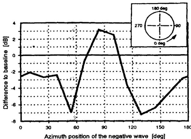
Fig. 3.31 Variation of SPL for 2-per-rev IBC input function vs. the position of the maximum negative amplitude on the advancing side ( $0^\circ < \Psi < 180^\circ$ )
