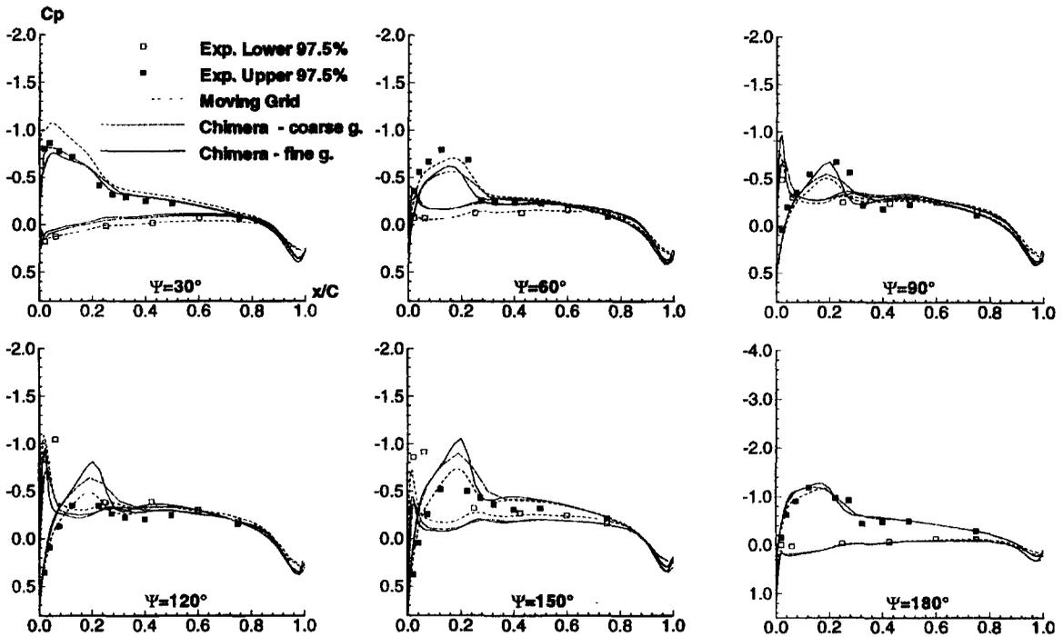
Fig. 3.17  $C_p$  distribution of the 7AD1 model rotor in high speed level flight at  $r/R = 0.975$  for different azimuth positions
