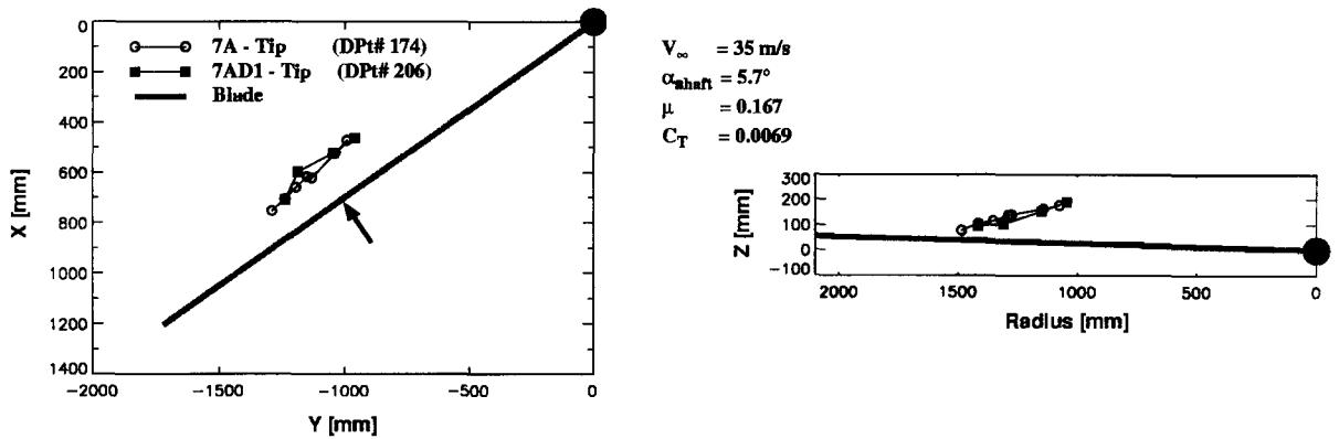
**Fig. 3.15** Vortex trajectories determined by LLS technique at a blade position of  $55^\circ$  azimuth for a moderate speed descent condition
