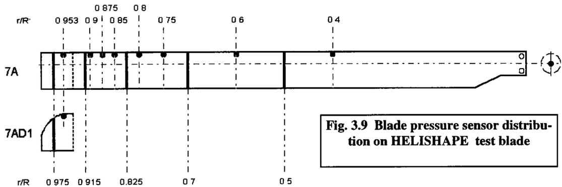
**Fig. 3.9 Blade pressure sensor distribution on HELISHAPE test blade**
