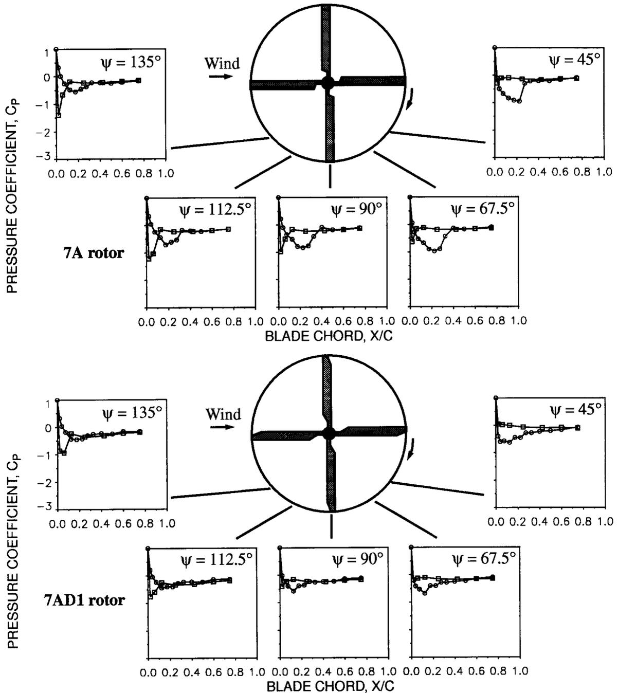
**Fig. 3.14 Typical chordwise blade pressure distributions at various blade azimuth locations for high speed flight at blade position  $r/R = 0.75$**
