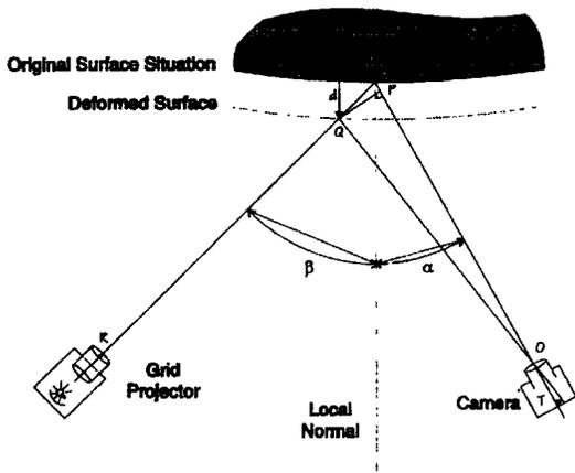
**Fig. 3.24 Principle of the Projected Grid Method (PGM)**
