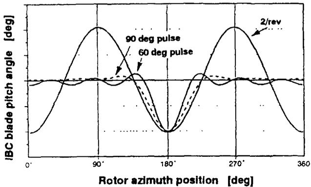
**Fig. 3.32 Definition of multi-harmonic input functions (pulse at blade root or wavelet at blade tip) compared to a 2-per-rev single frequency input function**
