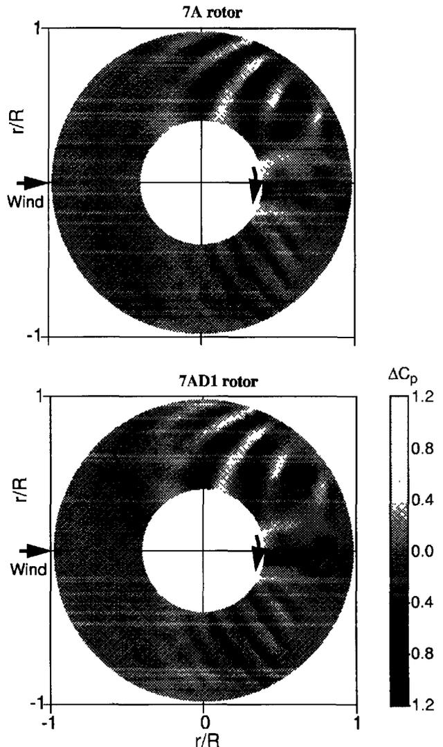
Fig. 3.13 Comparison of azimuthal /radial differential pressure distribution for the 7A and the 7AD1 rotor at moderate speed descent
