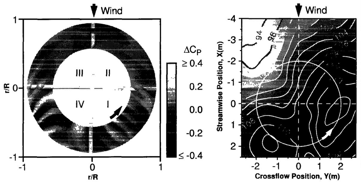
**Fig. 3.3** Blade surface pressure contour plot during one rotor revolution (high-pass filtered) for several sensors near the leading edge (left); corresponding acoustic radiation in terms of sound pressure level isobars below the rotor (right) for a moderate speed descent flight condition with strong BVI
