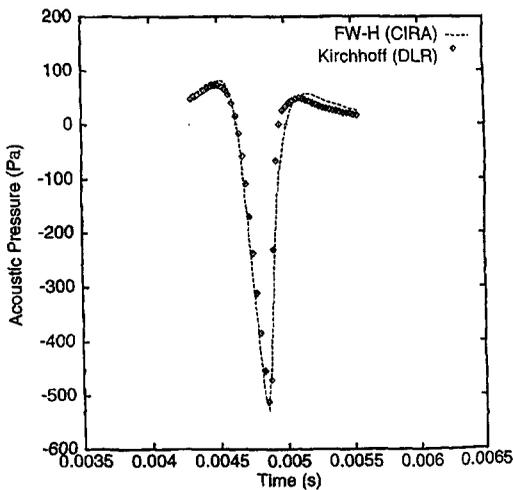
Regarding rotor acoustic radiation for a high speed rotor situation (without shock delocalisation), a typical result of the theoretical HELISHAPE effort appears in Fig. 3.18. Here results derived from (a) the acoustic analogy approach and (b) a Kirchhoff integral formulation with a CFD derived near-field close to the rotor indicate good agreement of both approaches.
