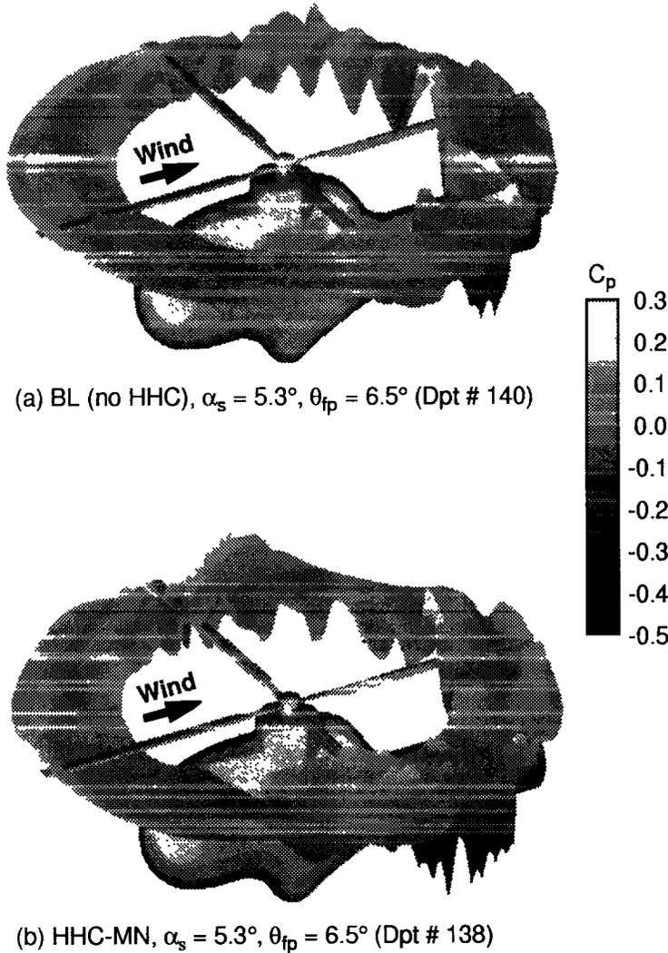
**Fig. 3.22** Upper surface leading edge blade pressure  $C_p$  distribution near the leading edge (at  $x/c = 0.03$ ) for low speed descent base line cases without and with HHC for minimum noise
