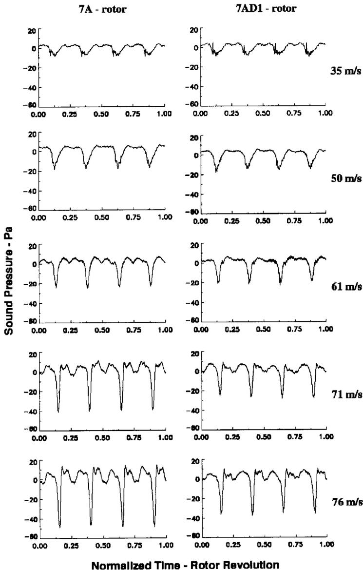
**Fig. 3.11 Comparison of 7A and 7AD1 in plane noise signatures in level flight for different flight speeds**
