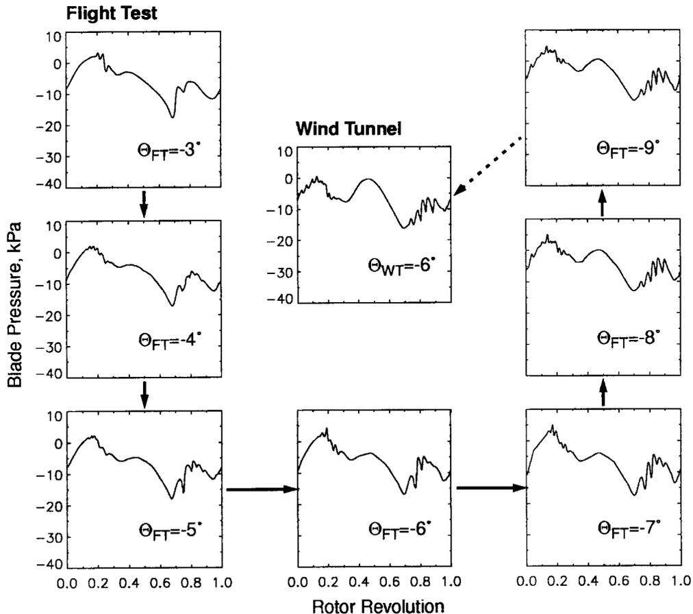
**Fig. 3.34 Comparison of blade pressure time histories for flight path angles ranging from  $-3^\circ$  to  $-9^\circ$  with one obtained in the wind tunnel at  $-6^\circ$  for conditions of moderate speed descent with strong BVI**
