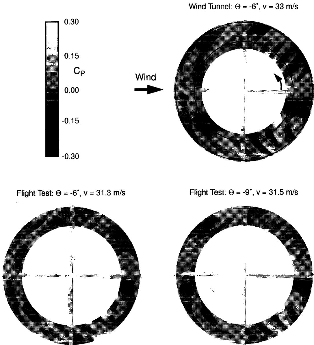
**Fig. 3.35 Blade pressure contour plots generated from upper surface leading edge sensor data for a moderate speed descent condition with strong BVI**
