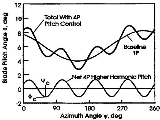
**Fig. 3.19 Higher Harmonic blade pitch angle variation**
