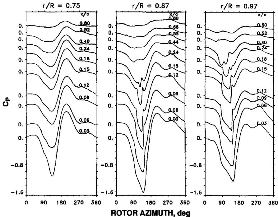
**Fig. 3.4** Averaged blade pressure time histories on the lower blade surface at different radial ( $r/R$ ) and chordwise ( $x/c$ ) locations for a high speed level flight condition
