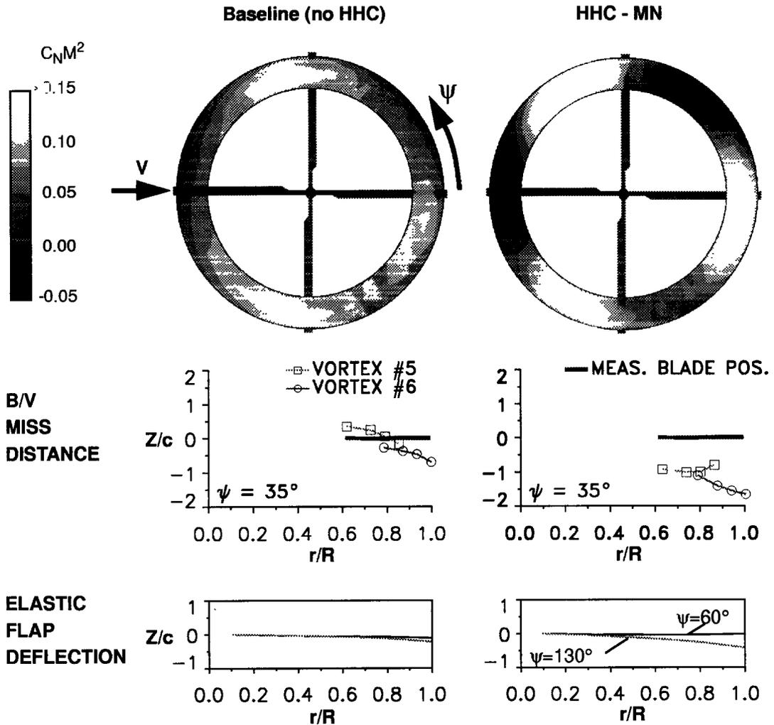
**Fig. 3.23** Effect of HHC on local normal force distribution on the rotor disk, on blade vortex separation distance and on elastic blade deformation at the locations of vortex emission ( $\psi = 130^\circ$ ) and vortex interaction ( $\psi = 60^\circ$ ) for the base line case and with HHC
