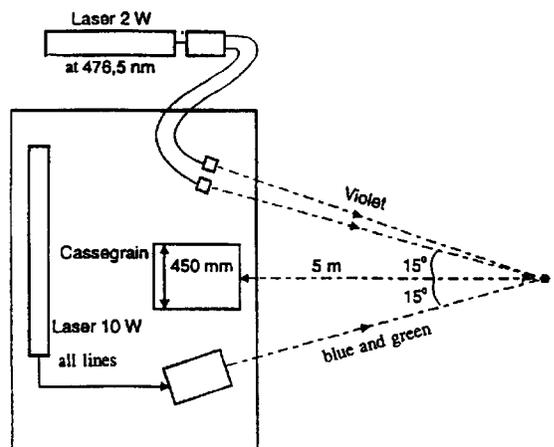
**Fig. 3.26 Schematic of 3-D LDV system**
