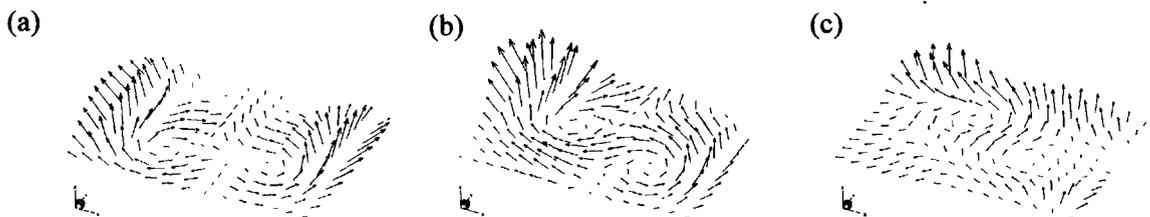
Fig.5. Calculated active sound intensity vectors on the measurement field plane at 508 Hz. (a) set 1, (b) set 2, (c) set 3.
