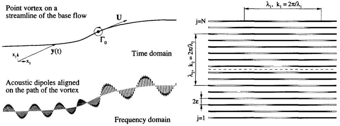
**Figure 1:** Illustration of the basic approach: spectral decomposition of moving point vortex (left),  $N$  vorticity waves with harmonically varying vorticity (right).
