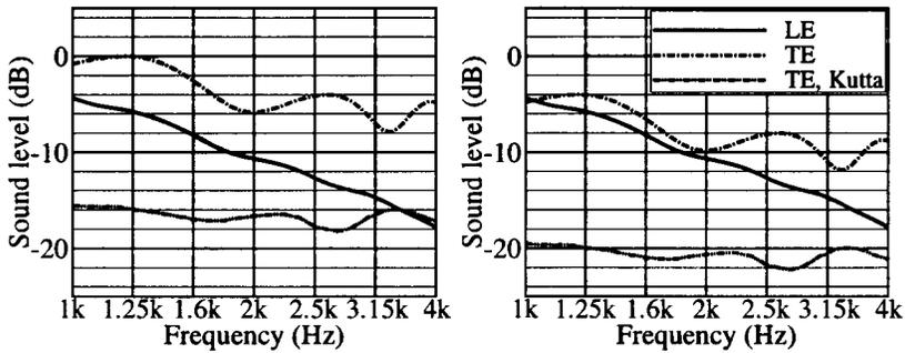
**Figure 4:** Predicted sound level from leading and trailing edge; FX-79-151A;  $M_0 = 0.18$ .
