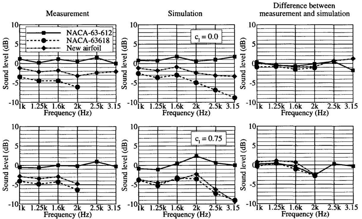
**Figure 5:** Measured and predicted sound levels for three different airfoils and two lift coefficients;  $M_0 = 0.18$ .
