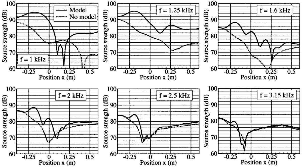
**Figure 3:** Acoustic image for different frequencies; FX-79-151A;  $M_0 = 0.18$ .
