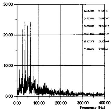
Fig. 6 Power Spectrum of the Aerodynamic Force
