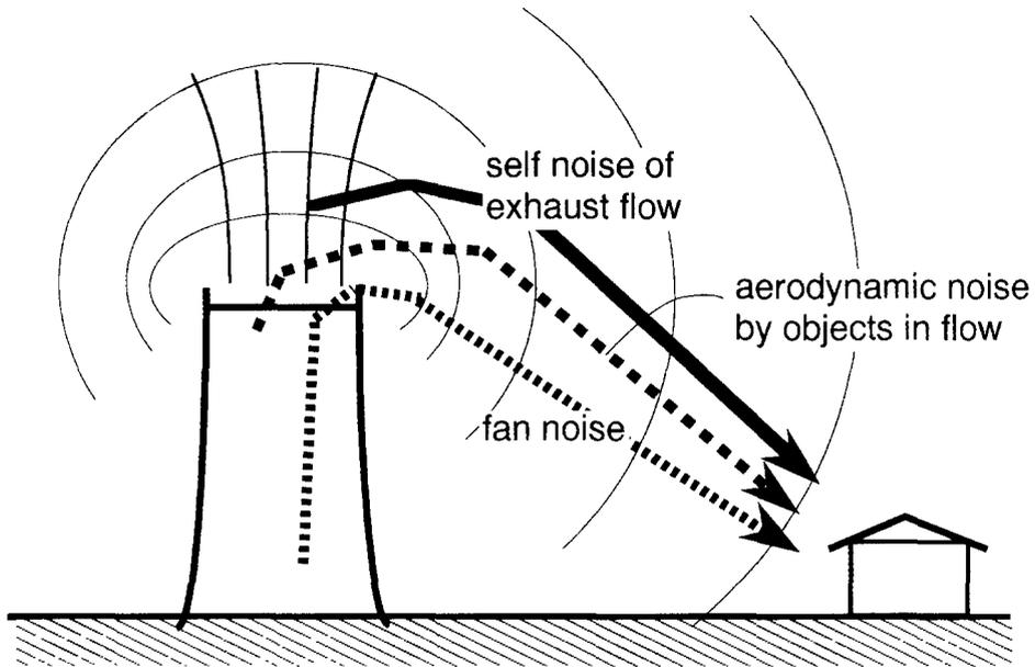
Fig. 1 Noises heard around a ventilation tower usually contain several noises.
