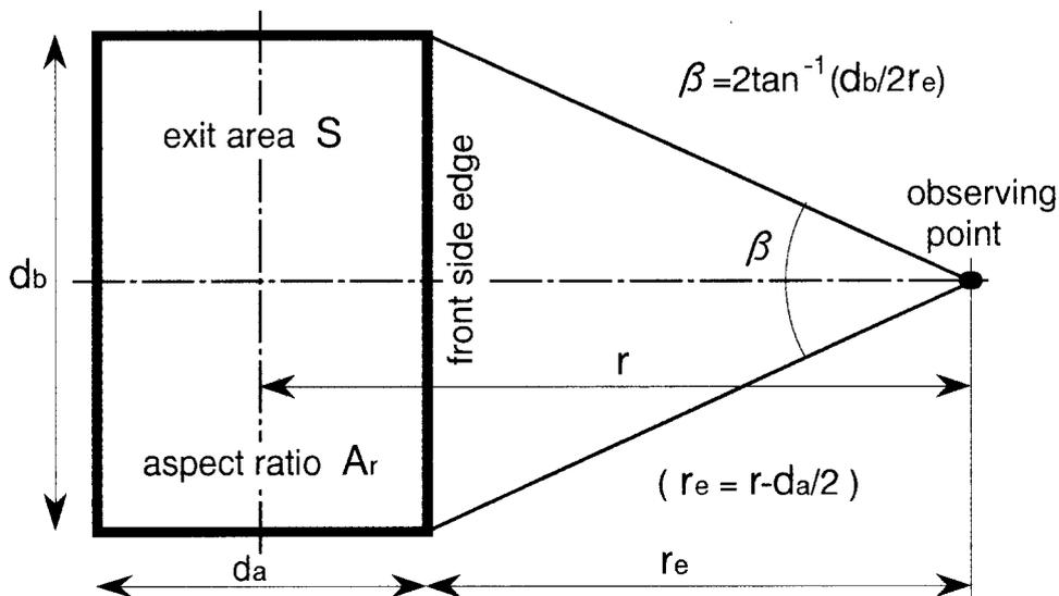
Fig. 10 Configuration of typical sizes around the exit used for estimations.
