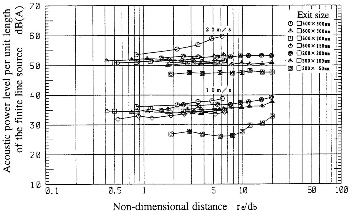
Fig. 9 Noise source powers calculated on the assumption of the finite line source were also nearly constant for the rectangular exit cases.
