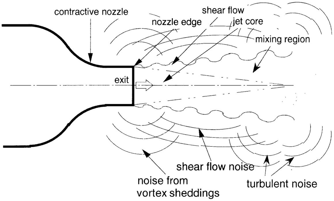
Fig 6 The blown out flow from a nozzle ordinaryly generats three kinds of aerodynamic sound sources.
