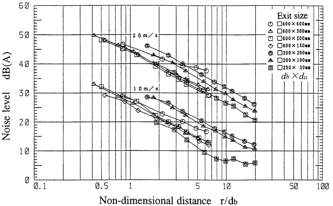
Fig. 7 Exhaust flow noise decreases almost constant by the non-dimensional distance normalized by the front side length of retangular exit.
