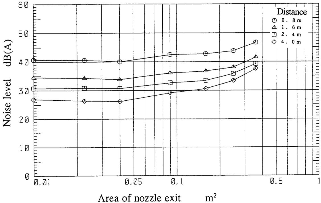
Fig. 5 Noise pressure changed with non-linear function of exit areas. (at exhaust flow velocity 20m/s, in the direction of perpendicular to the flow)
