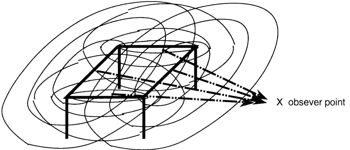
Fig. 8 The assumption that the shape of noise source was regarded as the finite line on exit side of the ventilation tower was suggested by the consideration of experimental results.
