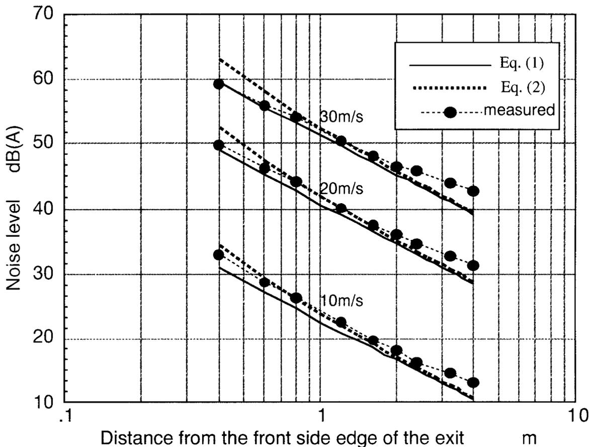
Fig. 11 Examples of estimated noise radiated from exhaust flows (exit type 600 x 300).
