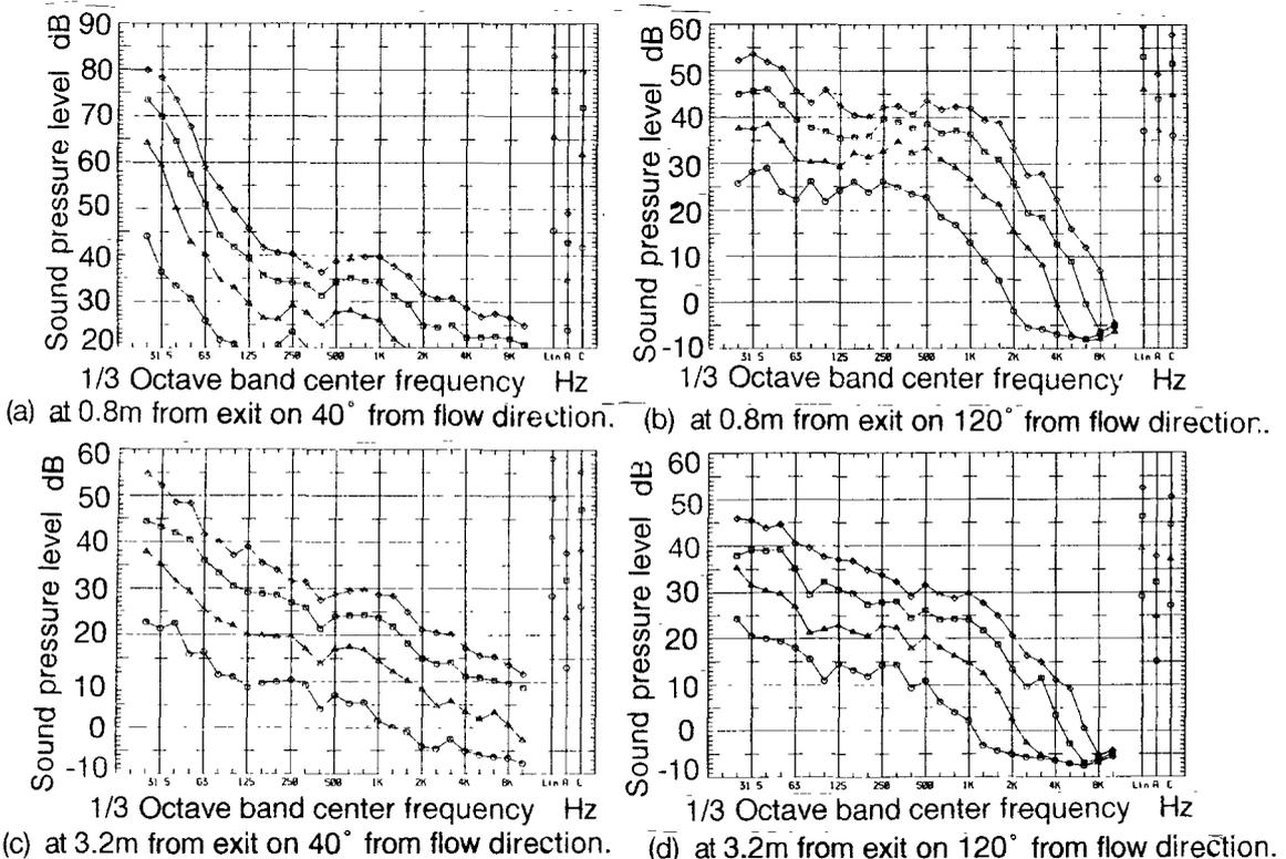
Fig. 4 Noise spectra at typical positions change with flow velocity
