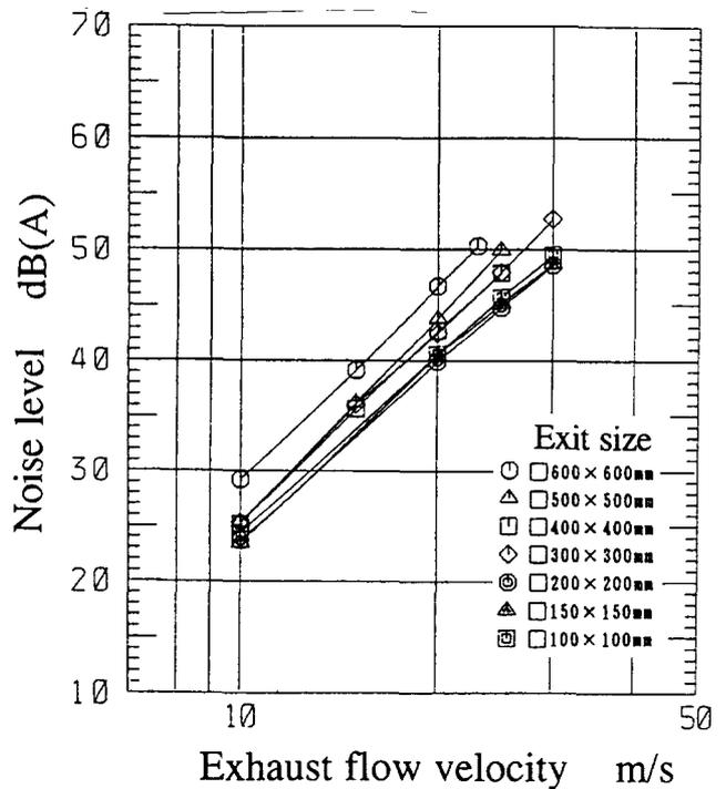
Fig. 3 The measured noise power was proportional to the 6th power of gas flow velocity.
