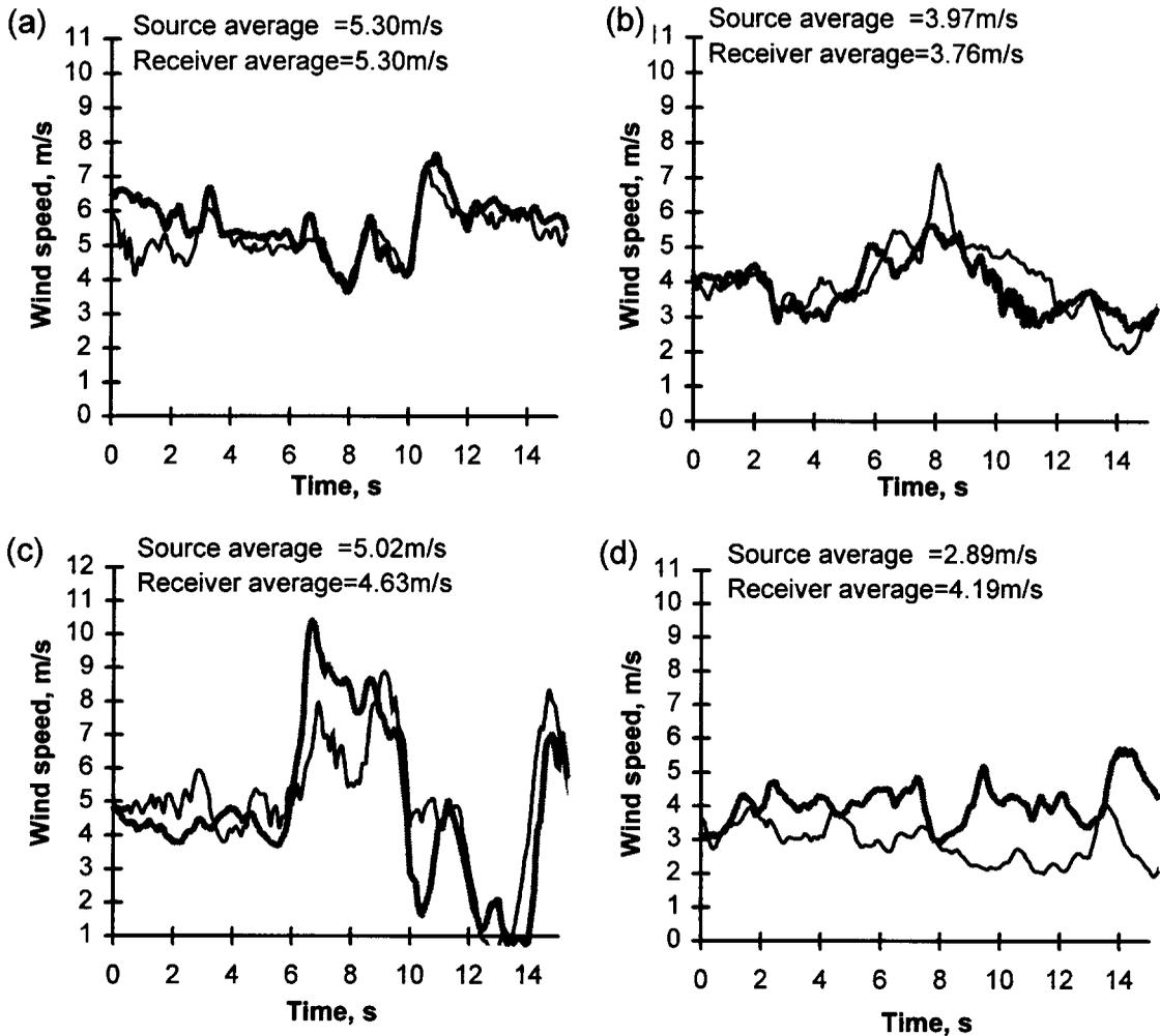
**Fig. 1 Comparison of wind speed time traces for four cases determined from anemometer readings at the source, thin lines, and at the receiver, thick lines.**
