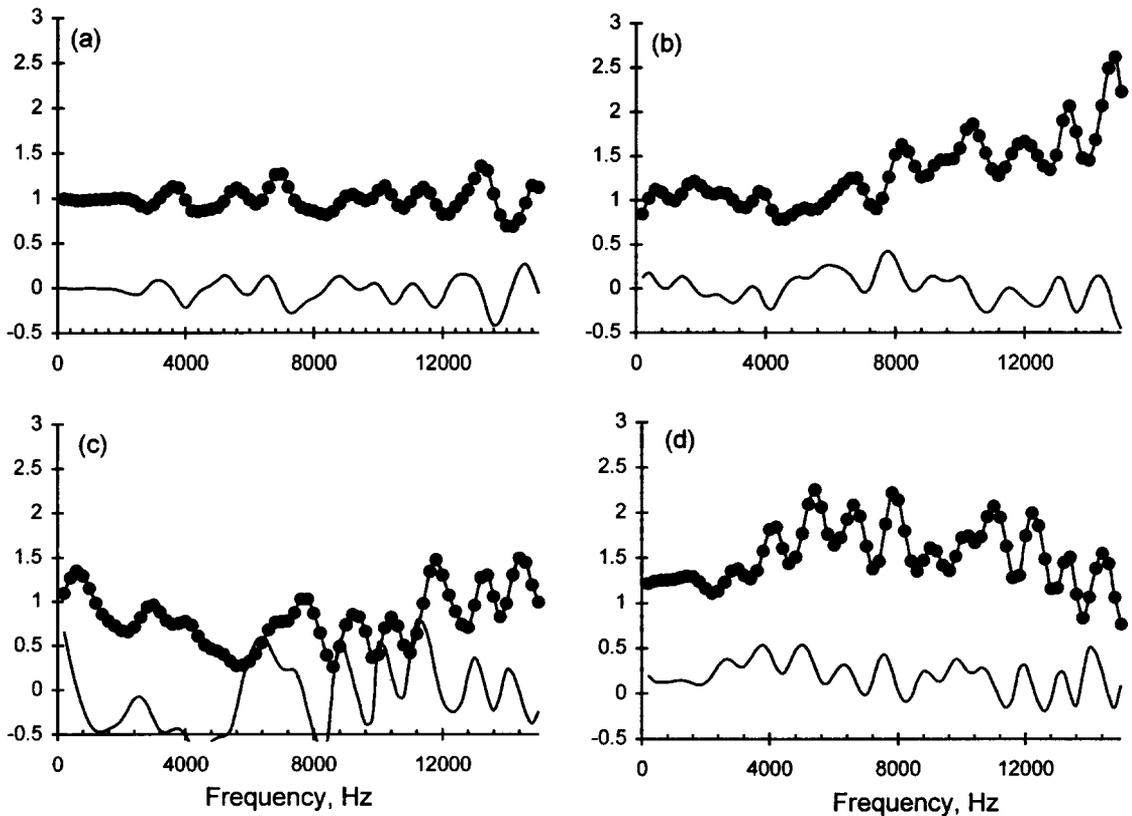
**Fig. 3 Transfer functions for (a) an indoor pulse and (b) to (d) outdoor pulses. The dots represent amplitude information while the thin lines are the phase variation.**
