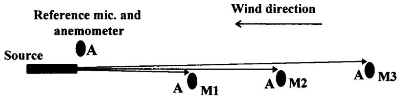
**Fig. 4 Plan view of the microphone and anemometer positions used in the array experiment.**
