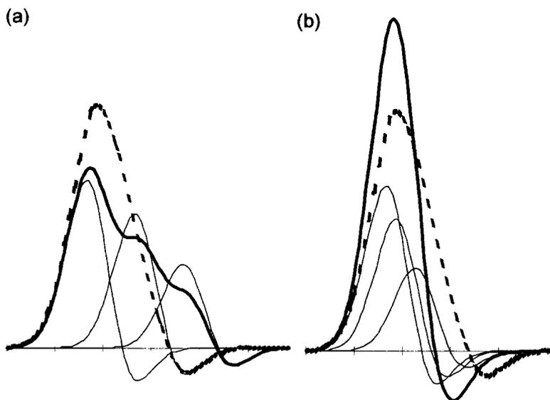
**Fig.7. Examples of the three pulselet model: (a) where the arrival time of each pulselets has increased resulting in a wider, reduced height pulse than the norm shown dashed, and (b) where reduced delays have resulted in a narrow, enhanced pulse.**
