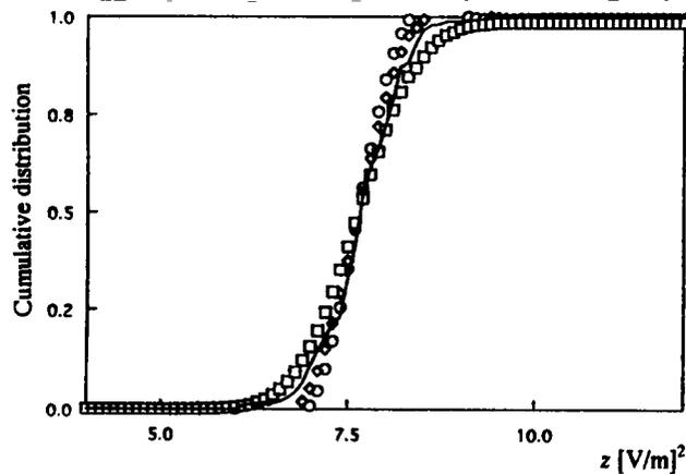
Fig.5 A comparison between the theoretical curves by use of the proposed precise estimation method and the experimental curve of cumulative distribution for the EM data. — : experimental curve. Theoretical values :  $\square$  first term ;  $\diamond$  first approximation ;  $\circ$  second approximation.
