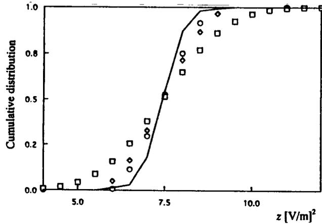
Fig.4 A comparison between the theoretical values by use of the unified probability expression and the experimental curve of cumulative distribution for the roughly observed EM data. — : experimental curve. Theoretical values :  $\square$  first term ;  $\diamond$  first approximation ;  $\circ$  second approximation.
