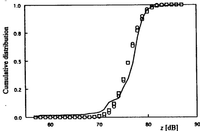
Fig.3 A comparison between the theoretical values by use of the proposed precise estimation method and the experimental curve of cumulative distribution for the sound level data. — : experimental curve. Theoretical values : □ first term ; ○ third approximation.
