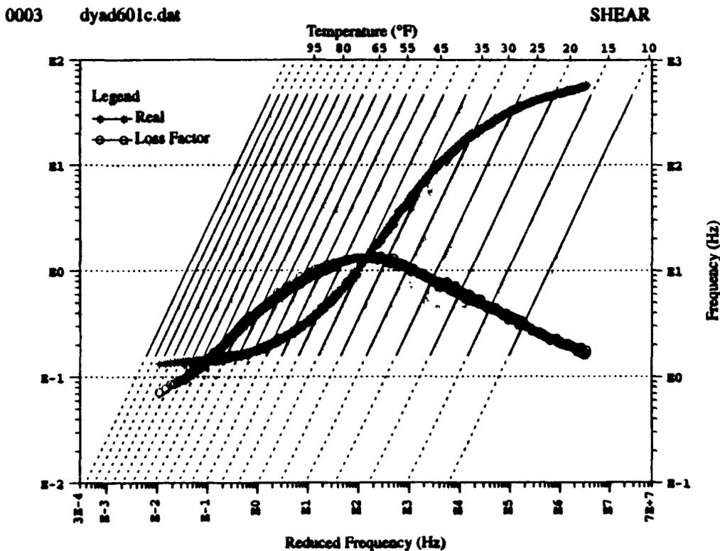
FIGURE 1 Loss factor as a function of frequency and temperature
