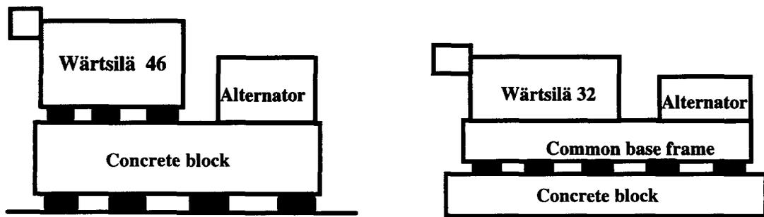
Figure 1: The sketches of the two most typical aggregates.
