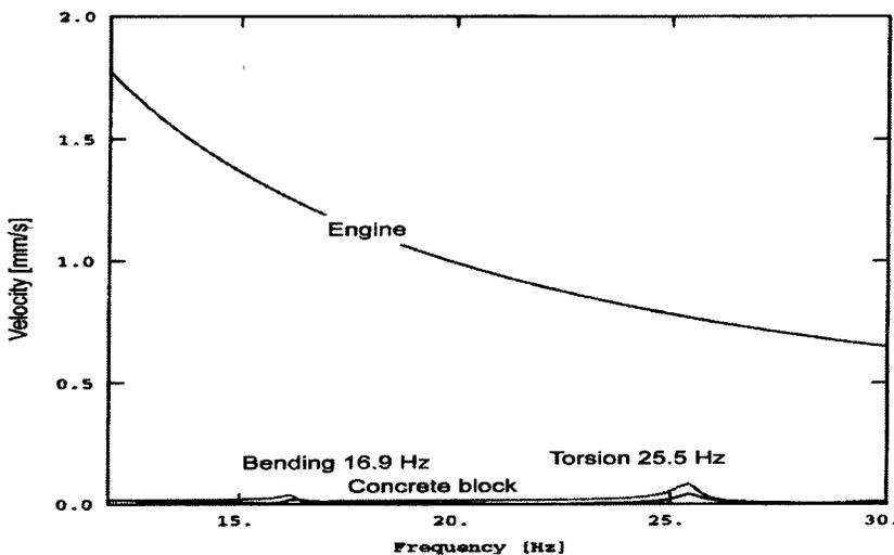
Figure 4: The vibration levels at the corner of the engine and the concrete block at frequency range 10 Hz to 30 Hz at torque  $M = 60$  kNm.
