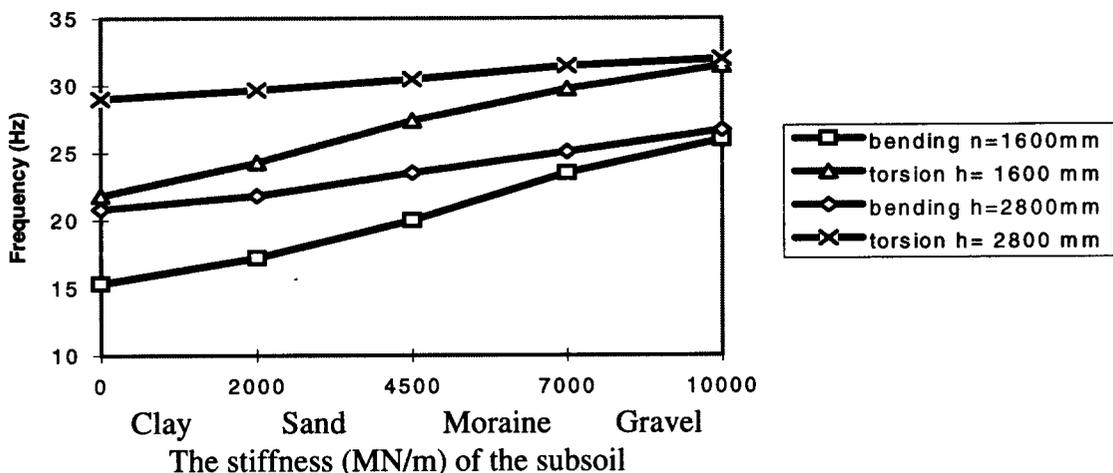
Figure 5: The influence of the subsoil for the lowest natural frequencies of the concrete block
