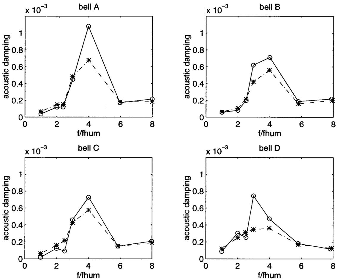
**Figure 3:** Measured (o) and calculated (\*) acoustic damping values.
