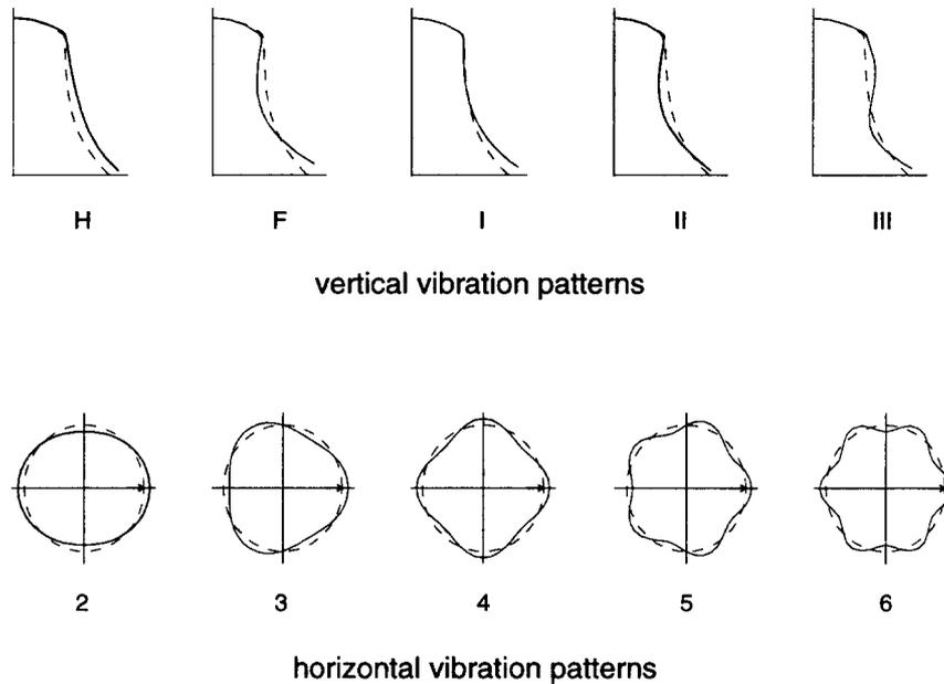
**Figure 1:** Vibration patterns of a bell.
