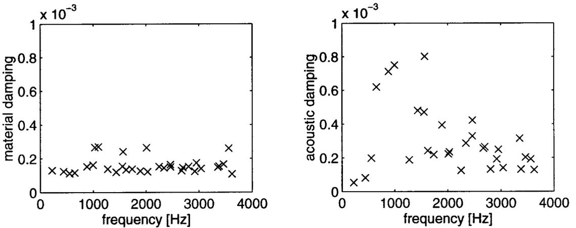
**Figure 2:** Measured damping values for bell B.
