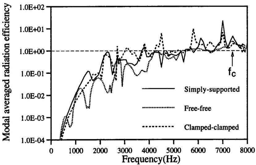
Fig.2. Radiation efficiency of an acoustically thick cylindrical shell
