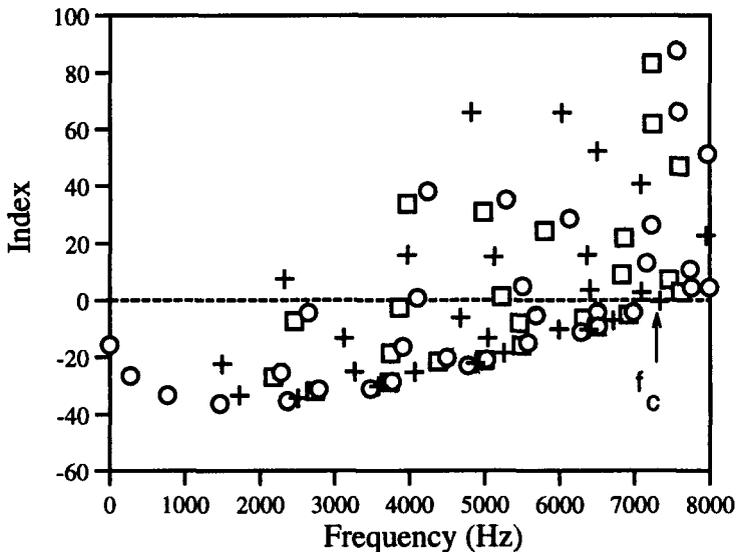
Fig.5. The index of each vibration mode of a cylindrical shell: +, simply-supported; o, free-free; square, clamped-clamped.
