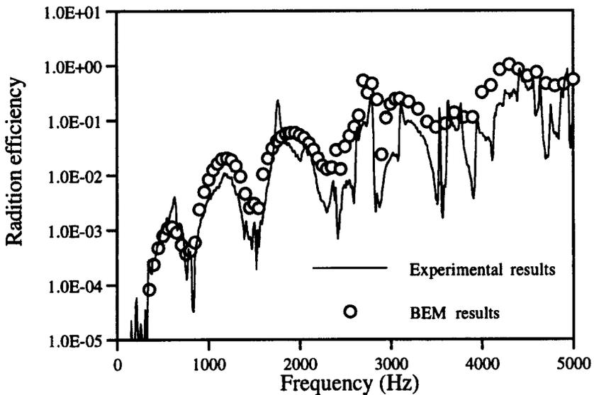
Fig.3 Comparison of the experimental results with BEM calculations
