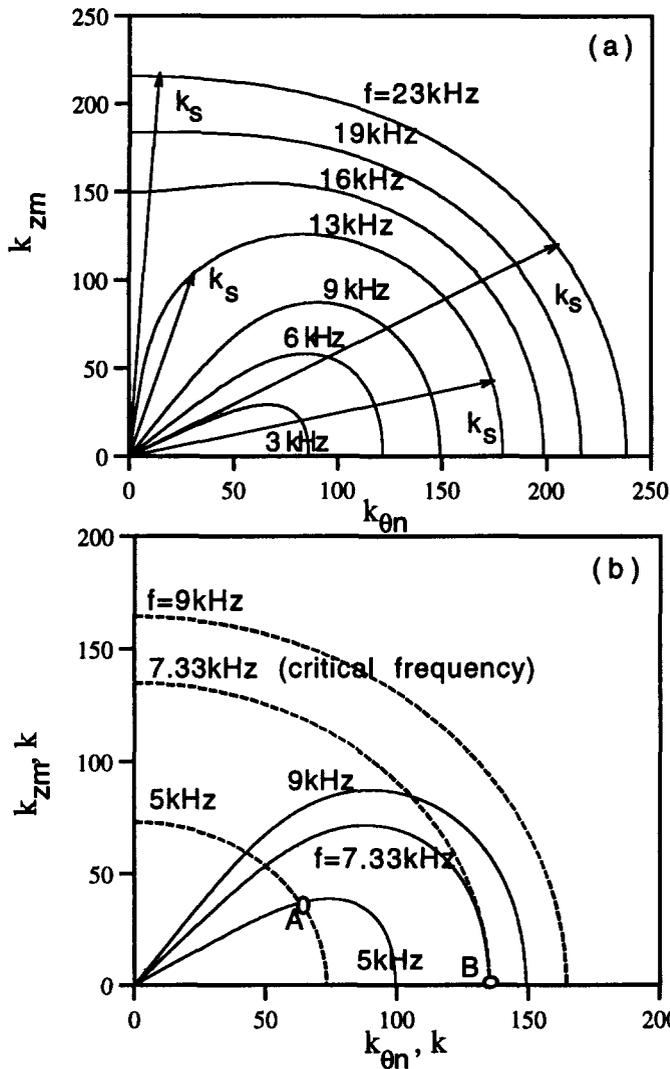
Fig.4. Wavenumber diagram for a cylindrical shell: ----, acoustic wavenumber; —, structural wavenumber;  $k_{\theta n}$ , circumferential structural wavenumber;  $k_{zm}'$ , axial structural wavenumber;  $k$ , acoustic wavenumber.
