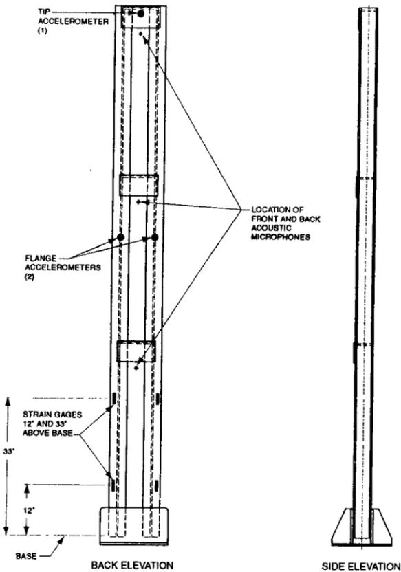
Figure 2. Test Article (Elevations)
