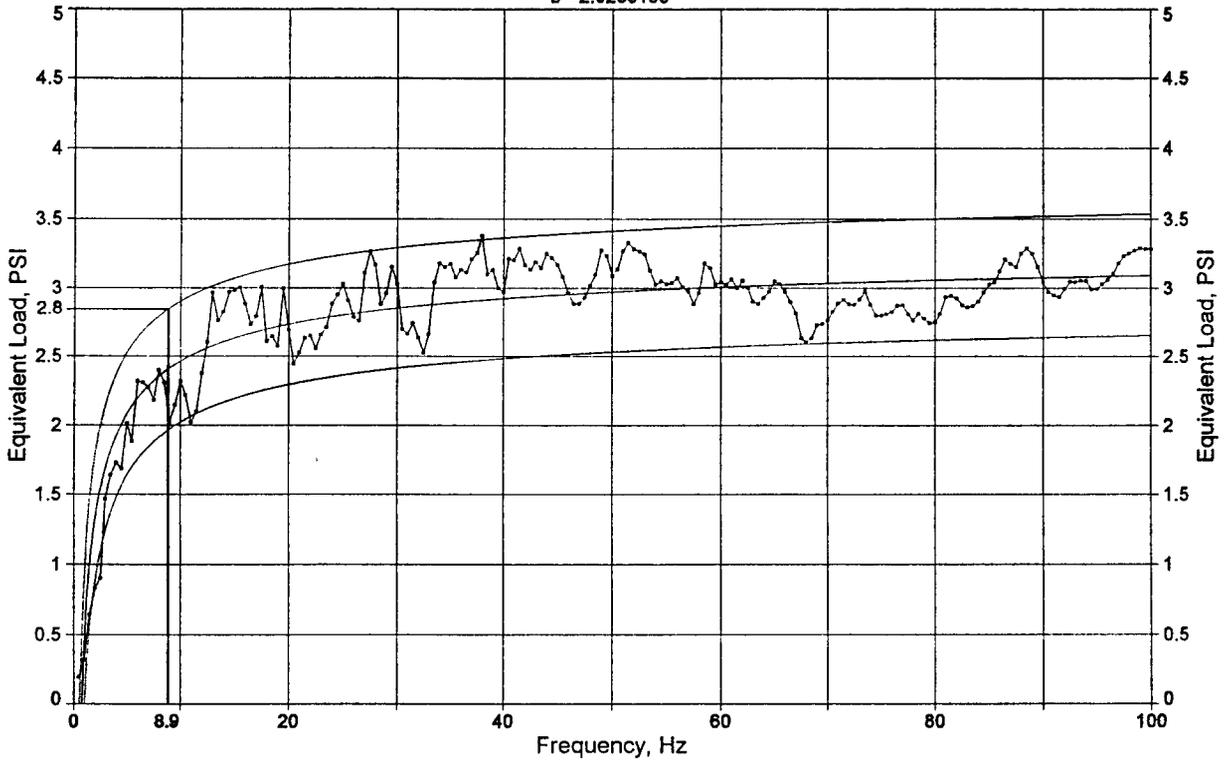
Figure 4. Response Spectra to Input Pressures (1 Percent Damping)
