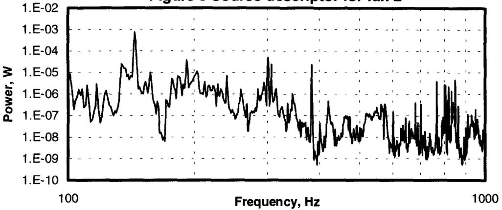
**Figure 4 Source descriptor for a central heating pump**
