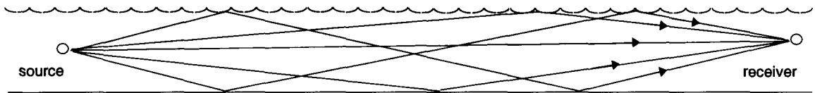
Figure 2: Sound transmission in an isovelocity shallow ocean
