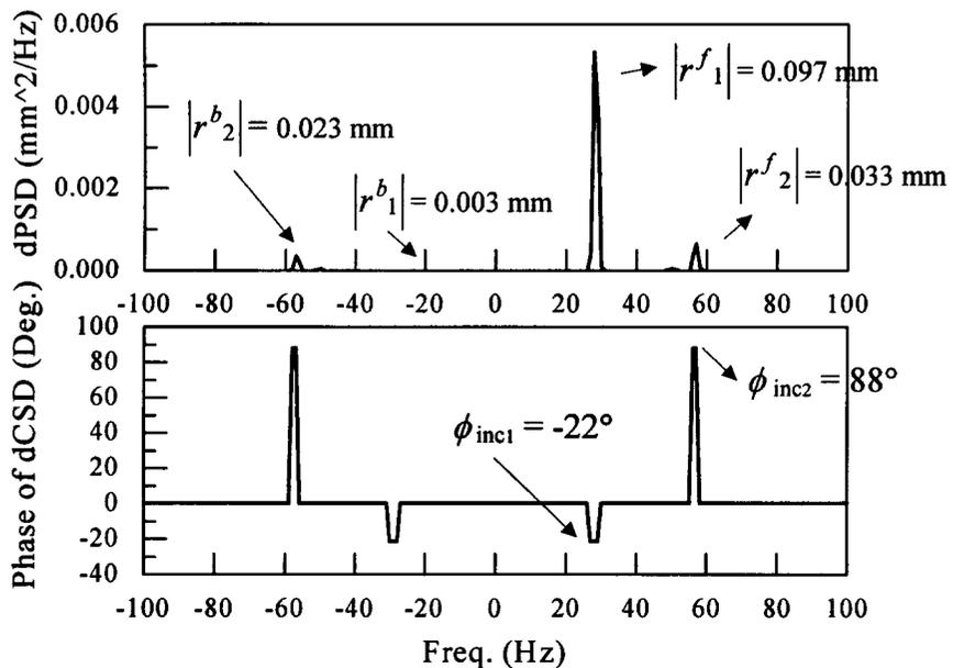
Figure 4 Directional power and cross spectra of complex-valued signal
