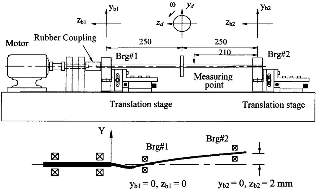
Figure 2 Experimental setup and type of angular misalignment ( $\Delta z_a = z_{b2} - z_{b1} = 2.0 \text{ mm}$ )
