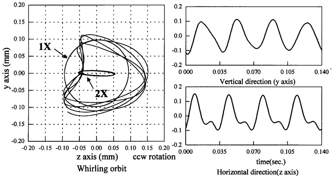
Figure 3 Whirling orbits and time histories at 1700 rpm:
