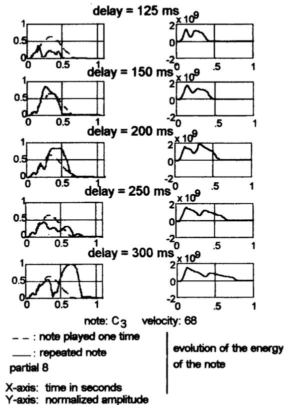
**Figure 4: Temporal evolution of partial #8 of note C<sub>3</sub> and the energy associated with this note in the case of repetition of the note.**
