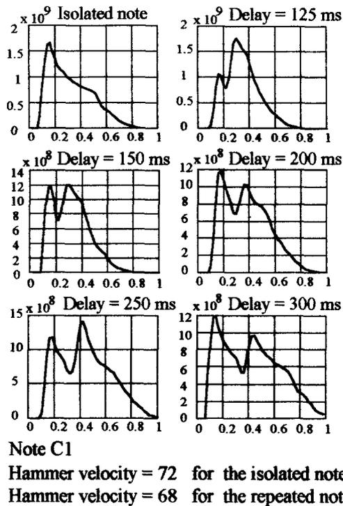
**Figure 2: Temporal evolution of the energy of note C<sub>1</sub> played twice successively with various delays.**
