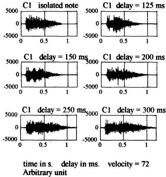
**Figure 1: Temporal signal of note  $C_1$  played twice successively with various delays. The second onset is not clearly visible in the different figures.**
