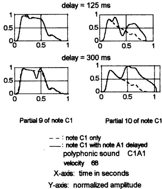
**Figure 5: Temporal evolution of partial #9 and #10 of note C<sub>1</sub> when notes C<sub>1</sub> and A<sub>1</sub> are played with a delay of 125 and 300 ms.**
