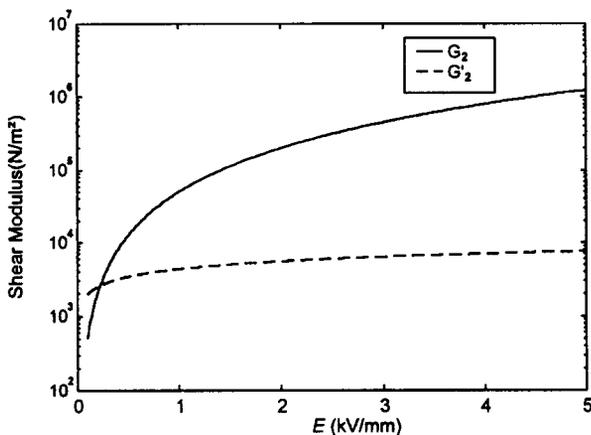
Figure 1. Shear Modulus of ER fluid
