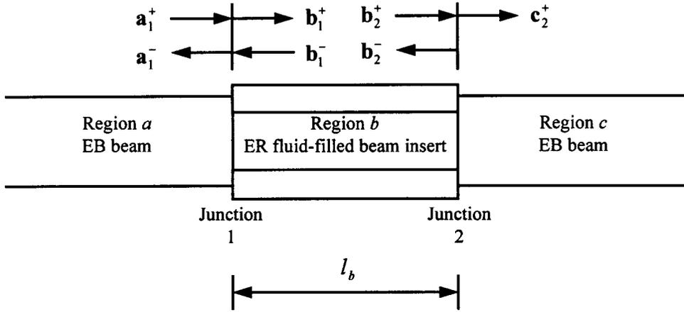
Figure 6. An ER fluid-filled beam insert in a Euler-Bernoulli beam and wave amplitudes.
