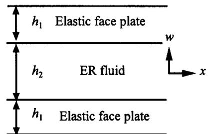
Figure 2. Diagram of ER Beam
