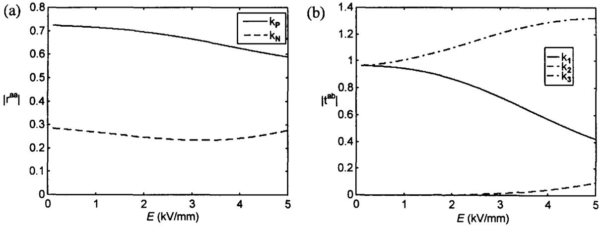
Figure 5. Magnitude of (a) reflection and (b) transmission coefficients for a propagating wave incident upon a junction between an Euler-Bernoulli and an ER beam,  $f=40$  Hz.
