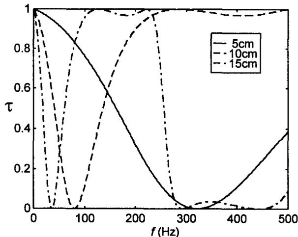
Figure 8. Transmitted power per unit incident power,  $\tau$ , for various lengths  $l_b$ ,  $E=2.5$  kV/mm.
