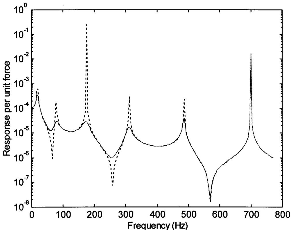
Figure 2. Frequency responses of the beam before (---) and after (—) wave control.
