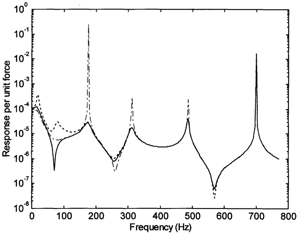
Figure 4. Frequency responses of the beam after wave (···), modal (-.-) and hybrid (—) control
