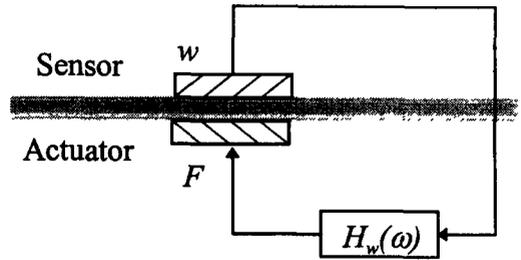
Figure 1. Collocated feedback control.
