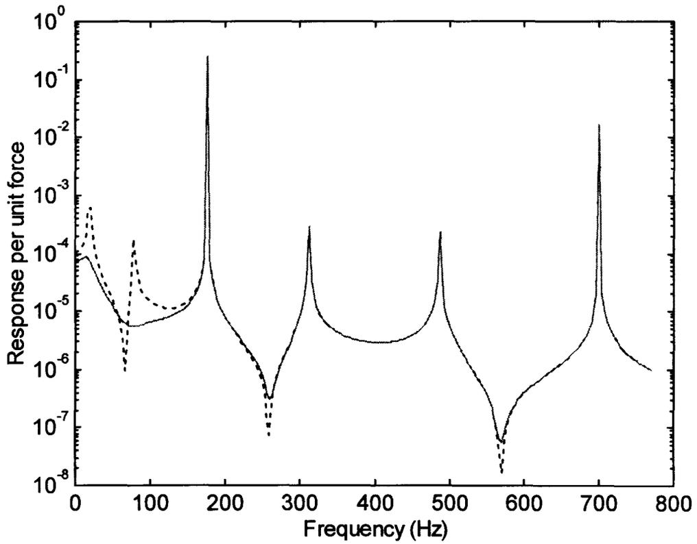
Figure 3. Frequency responses of the beam before (···) and after (—) modal control.
