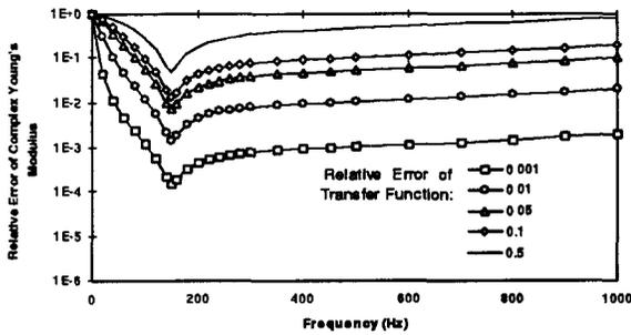
Fig.9 Error curve for the rod theory
