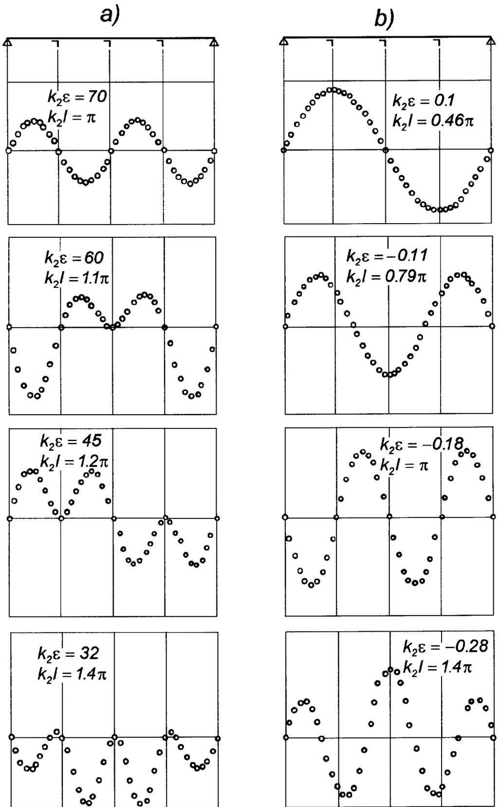
Fig.2. Forms of stiffened plate eigen-vibrations at high (a) and low (b) flexural rigidity of stiffeners (in comparison with rigidity of plates)
