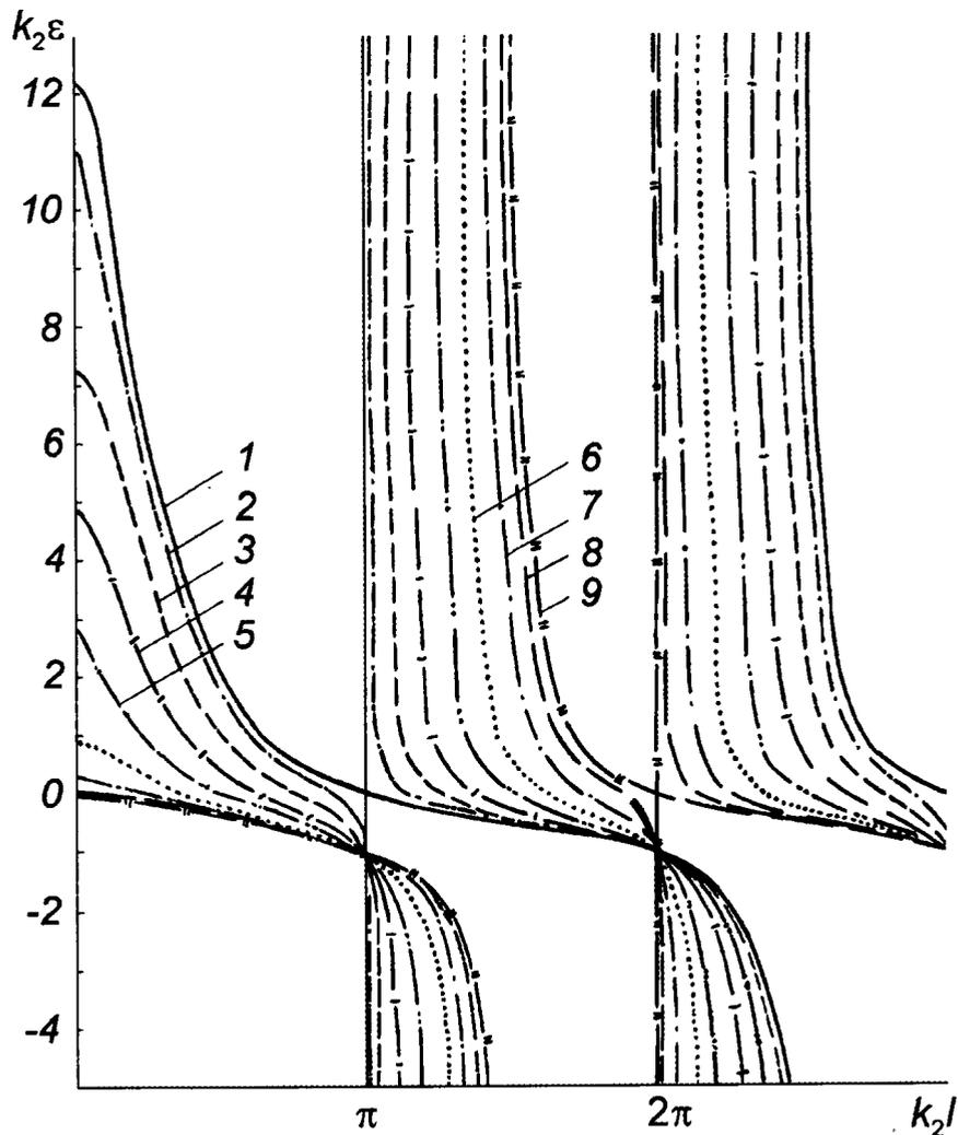
Fig.1. Effect of flexural rigidity of stiffeners on eigen-numbers of the stiffened plate: 1- $q/N=1.0$ ; 2-0.875; 3-0.75; 4-0.625; 5-0.5; 6-0.375; 7-0.25; 8-0.125; 9-0
