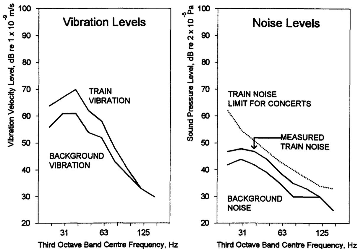
**Figure 5:** Measured vibration and noise levels in the stalls of the auditorium
