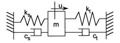
We now have just a single dof system, but with this system we can examine the effects of a support system on the elastic mode of the original two dof system. This model is even more useful because it also models the effects of an added constraint on the single dof system with a fixed boundary condition. This is a trivial model, but we can gain insight from its solution. The homogeneous differential equation is
