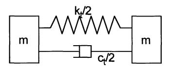
We could add support conditions in several ways, but let us add them symmetrically as diagrammed below. Here  $k_t$  and  $c_t$  designate the true stiffness and damping of the structure, while  $k_s$  and  $c_s$  designate the added support stiffness and damping.
