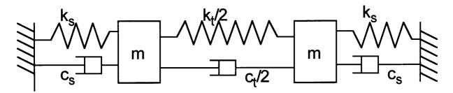
This system is a two degree-of-freedom system, but we are really only concerned with the effects of the supports on the elastic mode. Since that mode shape is symmetric, we can simplify the equations by cutting the dynamic system in half, and imposing a fixed boundary condition, as diagrammed below.
