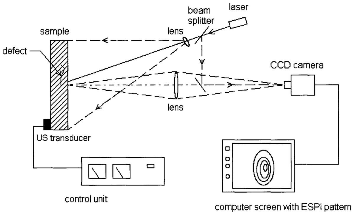
Fig. 1 - *Experimental setup: ESPI equipment for out-of-plane imaging of loss angle induced absorption of ultrasound emitted by transducer attached to sample*
