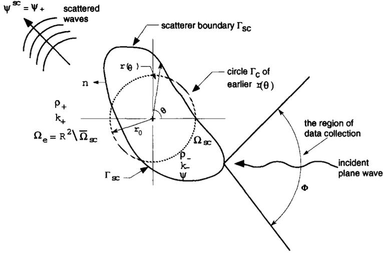
**Figure 1.** The geometry of scattering of a plane acoustic wave from an obstacle. The scatterer shape is given by  $r(\theta) = r_0 + \lambda f(\theta)$ ,  $\theta \in [0, 2\pi]$ .  $\Phi_0 \leq \Phi \leq 2\pi$ ,  $\Phi_0 > 0$ . For a Neumann object the interior wavenumber  $k_-$  vanishes.
