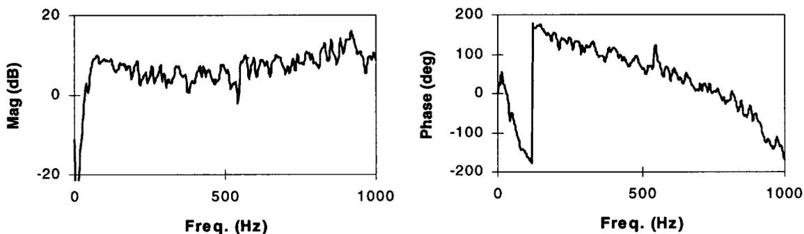
Fig.3. Measured open-loop frequency response of the uncompensated system in Example 1.
