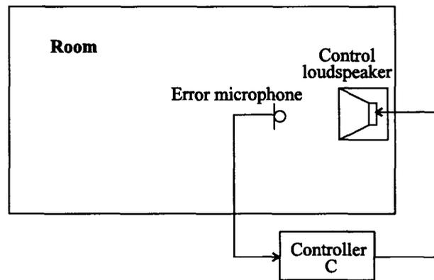
Fig.1. Feedback control system.
