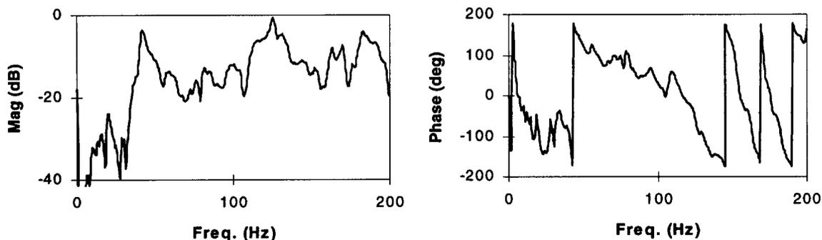
Fig.8. Measured open-loop frequency response of the uncompensated system in Example 3.
