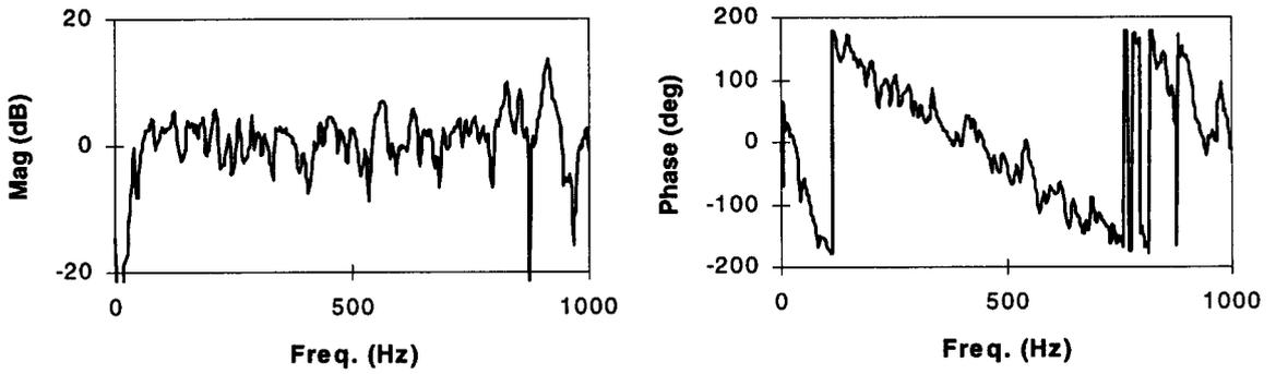
Fig.5. Measured open-loop frequency response of the uncompensated system in Example 2.
