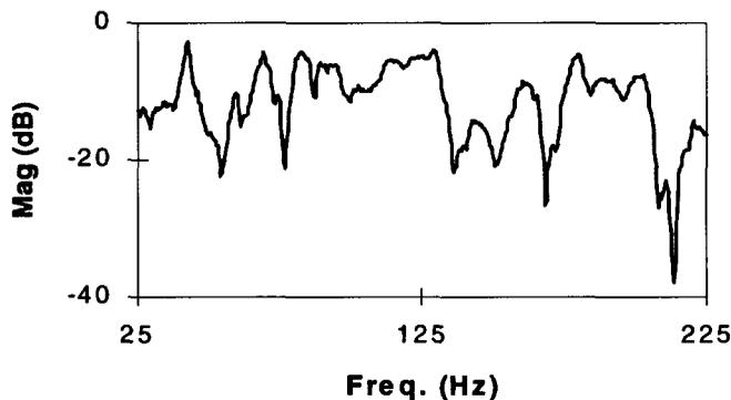
Fig.2. Typical acoustic frequency response of the room
