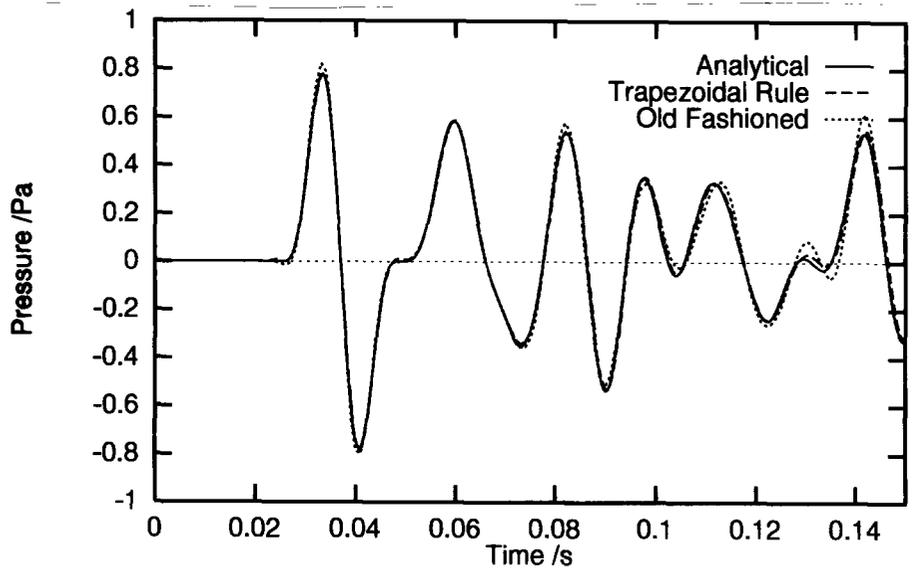
Figure 9: The response at (9,0,0) predicted by an analytical method and using FE-models based on two different discretisation principles.
