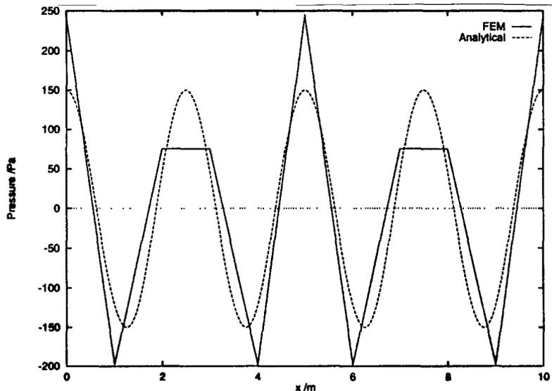
*Figure 1: The eighth non-trivial eigen mode in a 10m long hard 1-dimensional cavity calculated analytically and using an FE-model consisting of ten linear elements. Note that the error cannot be described as an overall error on wavelength.*
