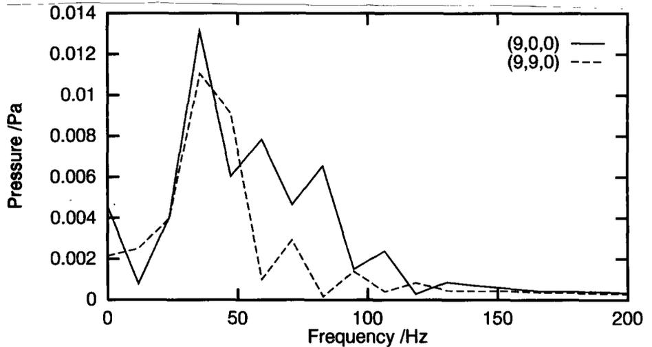
Figure 8: Amplitude spectrum of the first part of the response predicted with the central difference method at two different points.
