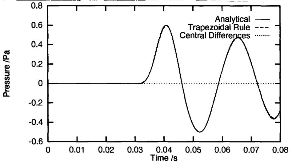
Figure 7: The response at (9,9,0) predicted with an analytical method and using FEM with two different time integration algorithms.
