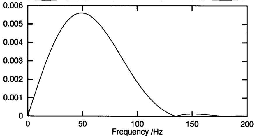
Figure 5: Amplitude spectrum of the excitation function.
