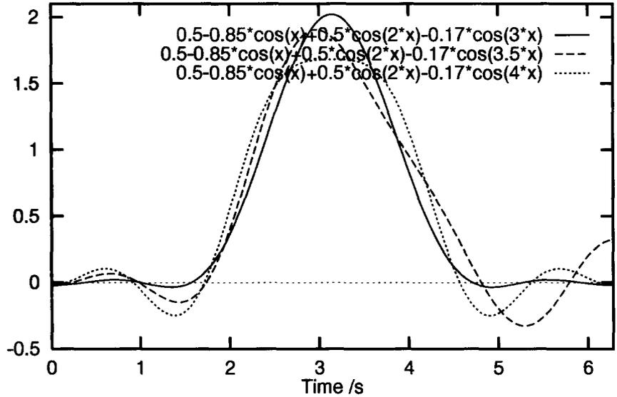
Figure 2: A function with different degrees of distortion on the highest frequency component. Illustrates the effect of phase errors from error on frequency.
