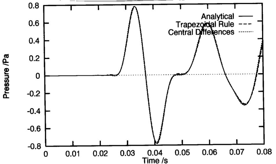
Figure 6: The response at (9,0,0) calculated using an analytical method and FEM using two different time integration algorithms.
