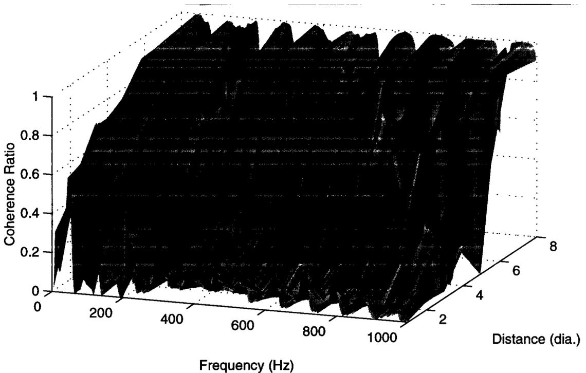
Figure 5 Coherence measured for 180° angular separations at 1, 2, 3, 4, 5, 6 and 8 diameters with the flanged pipe end condition
