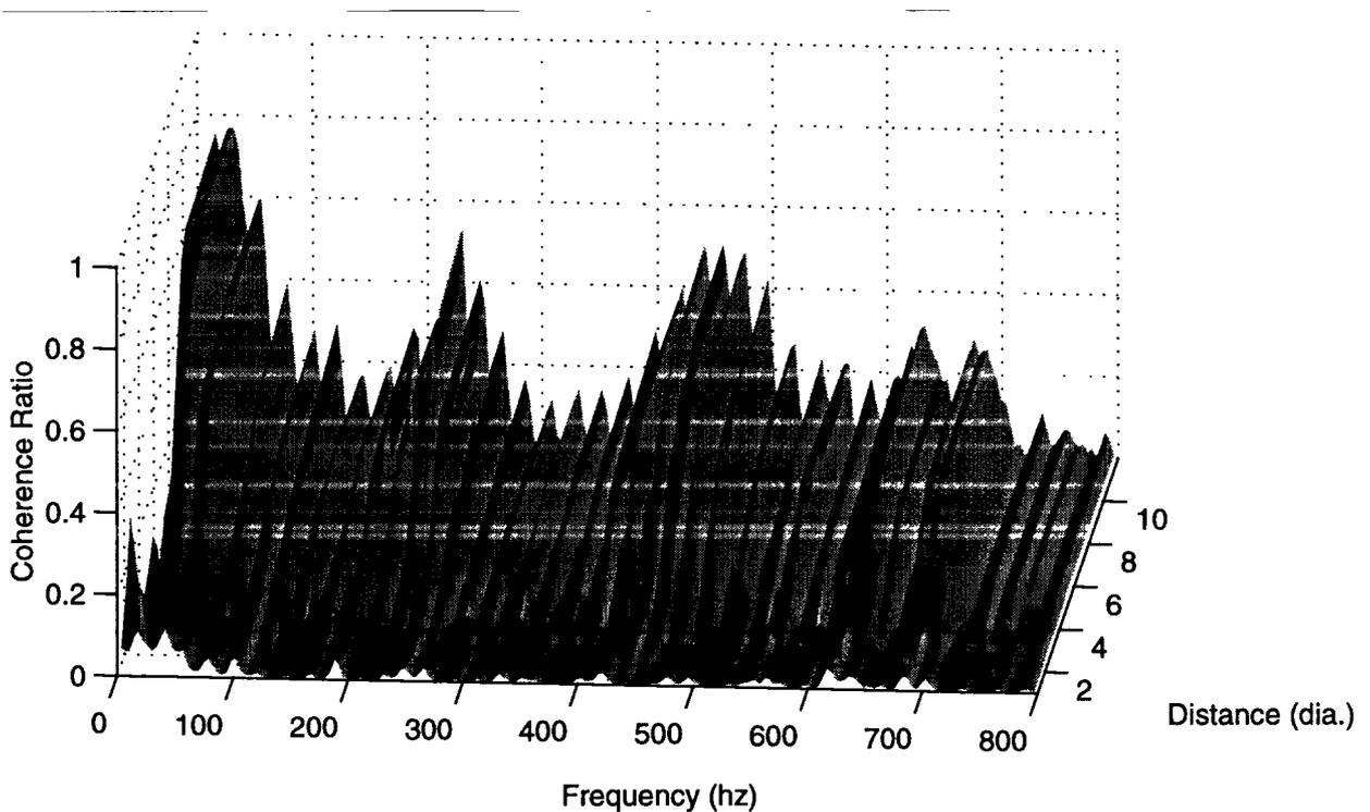
Figure 10 Coherence measured between -2 and 1, 2, 3, 4, 5, 6, 8 and 12 diameters with the anechoic termination end condition
