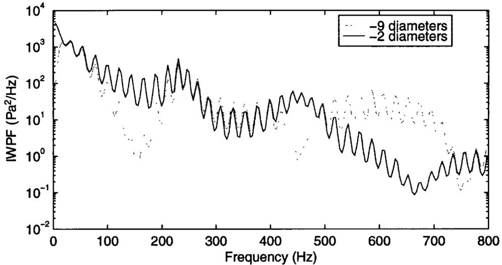
Figure 8 Typical autospectra at -9 and -2 diameters for 0 to 800 Hz
