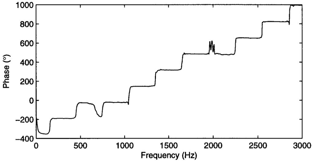
Figure 9 Typical unwrapped phase of the cross spectrum between -9 and -2 diameters
