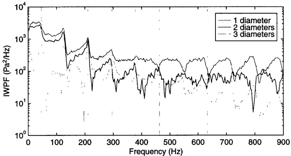
Figure 6 Cross spectra magnitudes of the internal wall pressure fluctuations (IWPF) at 1,2,3 diameters with the flanged pipe end condition
