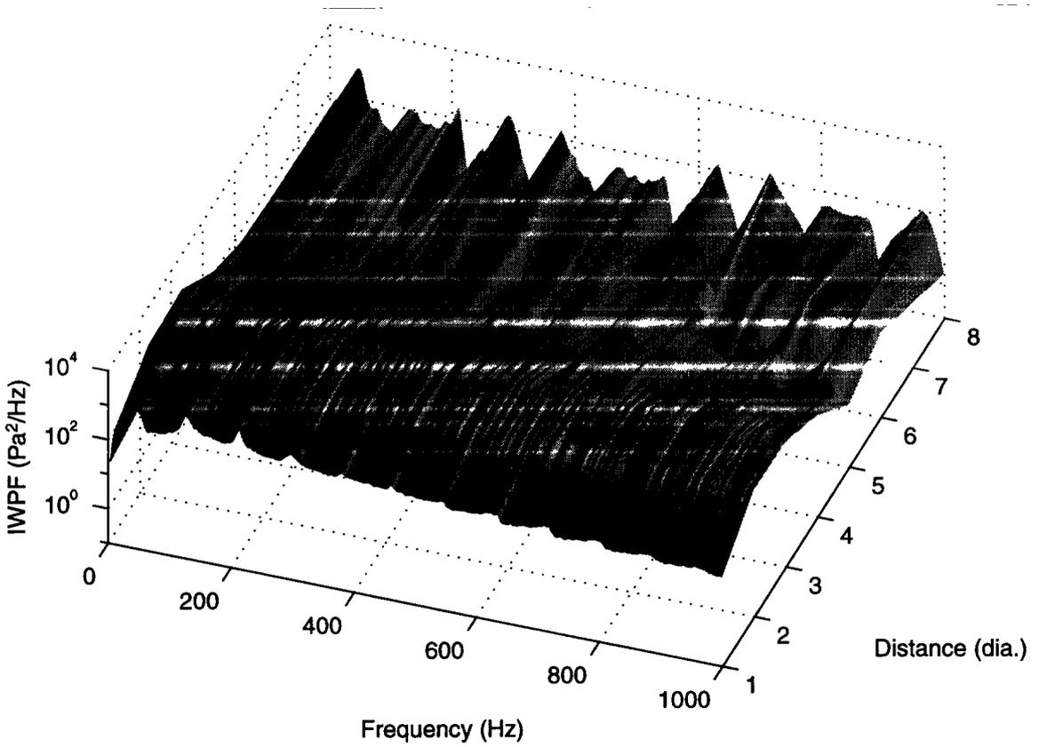
Figure 4 Autospectra of the internal wall pressure fluctuations (IWPF) measured at 1, 2, 3, 4, 5, 6 and 8 diameters with the flanged pipe end condition up to 1000 Hz
