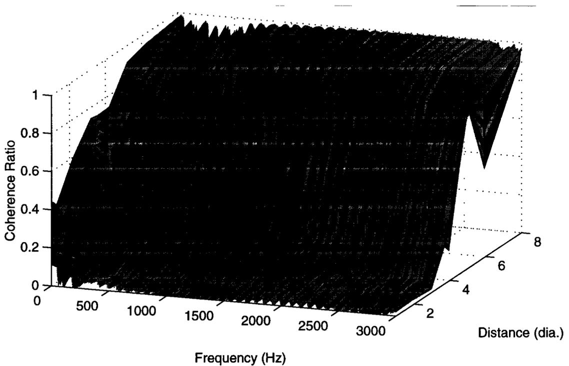
Figure 3 Coherence measured for  $180^\circ$  angular separations at 1, 2, 3, 4, 5, 6 and 8 diameters with the anechoic termination end condition
