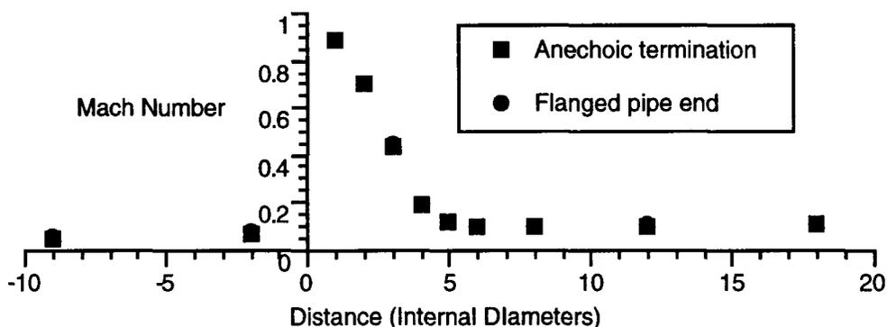
Figure 1 Mach numbers obtained from static and total pressure measurements at each axial location with a reference temperature at -2 diameters of 16°C for the 23 mm orifice
