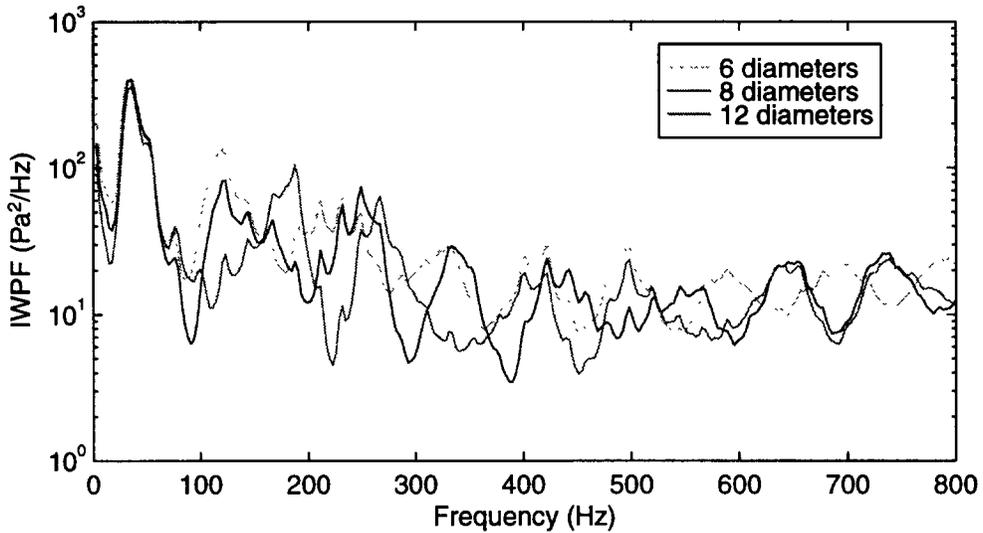
Figure 7 Autospectra at 6, 8 and 12 diameters for 0 to 800 Hz with anechoic termination end condition
