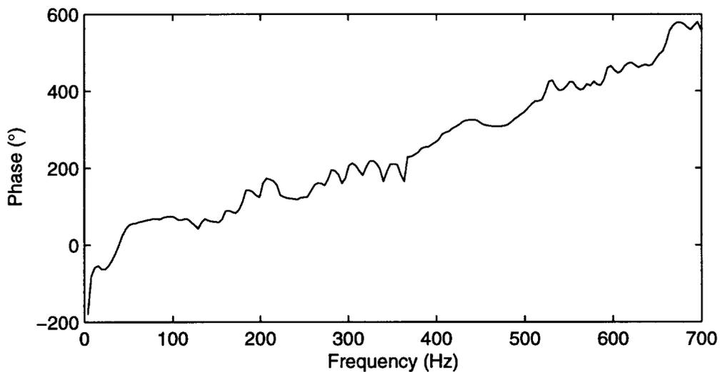
Figure 11 Unwrapped phase of the cross spectrum from -2 diameters to 12 diameters with the anechoic termination end condition
