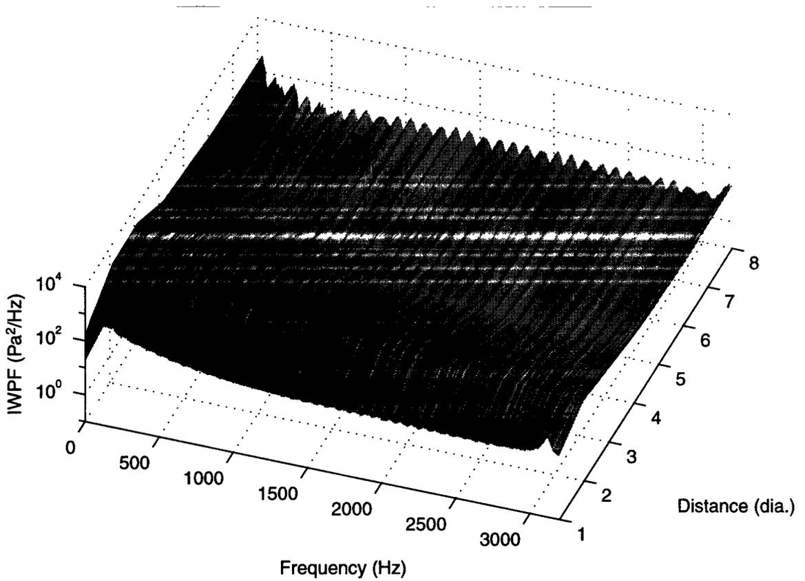
Figure 2 Autospectra of the internal wall pressure fluctuations (IWPF) measured at 1, 2, 3, 4, 5, 6 and 8 diameters with the anechoic termination end condition
