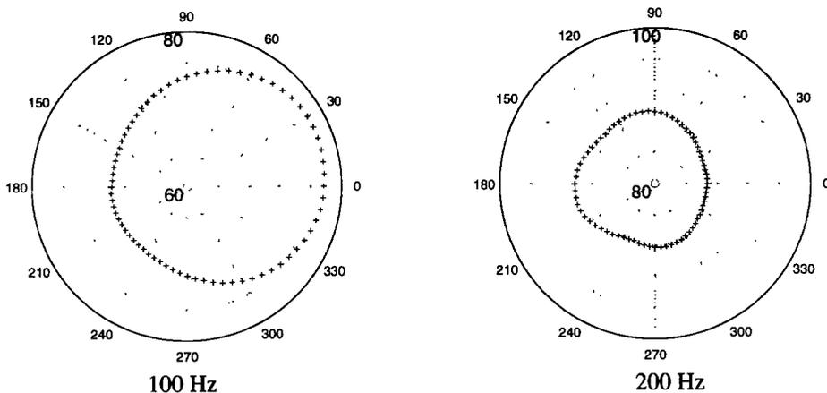
**Figure 8** Sound pressure level (dB) as a function of angular location  $\theta$ , with the microphone at 0.5 m
