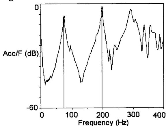
**Figure 4** Acceleration response of the curved panel with a backing cavity
