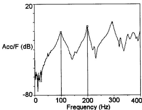
**Figure 6** Frequency response of the adjusted curved panel with backing cavity
