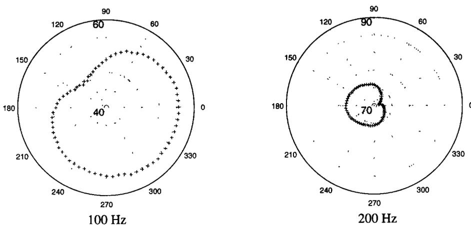
**Figure 9** Sound pressure level (dB) as a function of angular location  $\theta$ , with the microphone at 3.44 m
