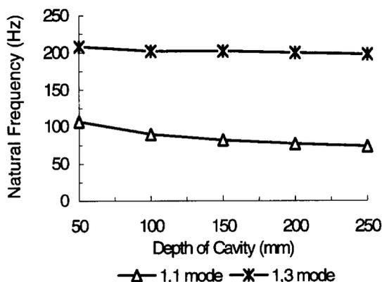
**Figure 5** The effect of variations in backing cavity depth on the panel resonance frequency
