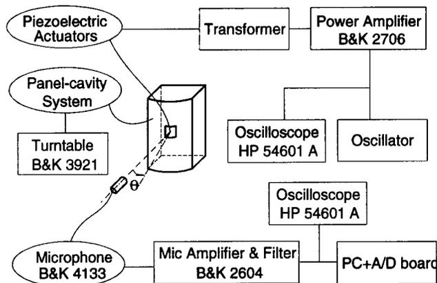
**Figure 7** Experimental set-up for sound radiation measurement
