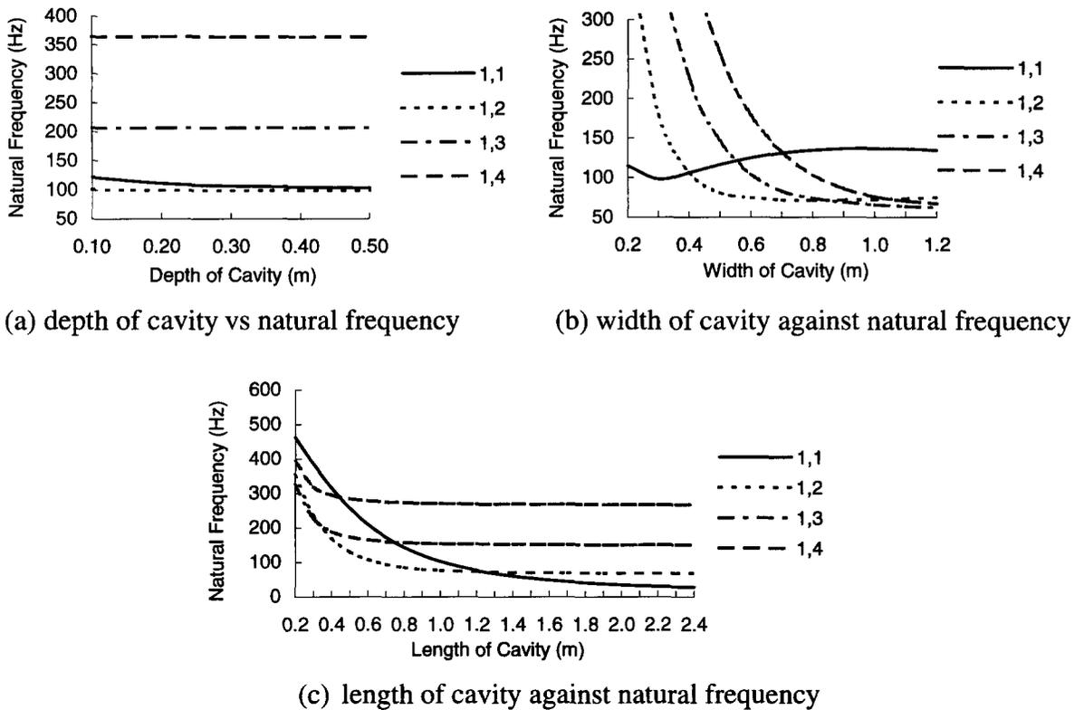
**Figure 3.** Variations of natural frequencies of the panel-cavity system as a function of cavity size
