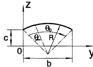
**Figure 1.** Curved panel with a backing cavity
